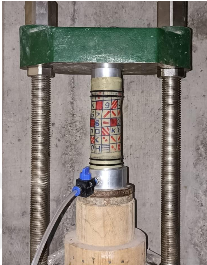
Figure 3. 4. A soil sample ready to be axially loaded by the jack
