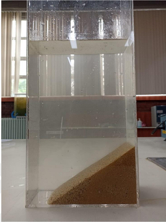
Figure 3. 18. Critical state angle of shearing resistance experiment performed on Sile Silica sand
