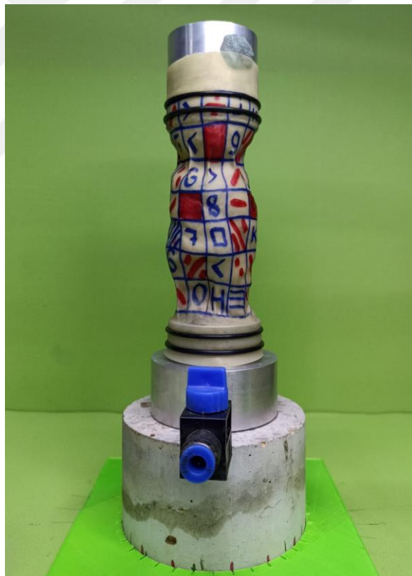
Figure 3. 6. View of marked membrane and reshaped sample
