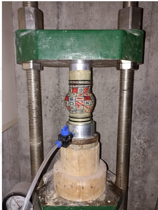
Figure 3. 5. Sample with over 40% axial deformation
