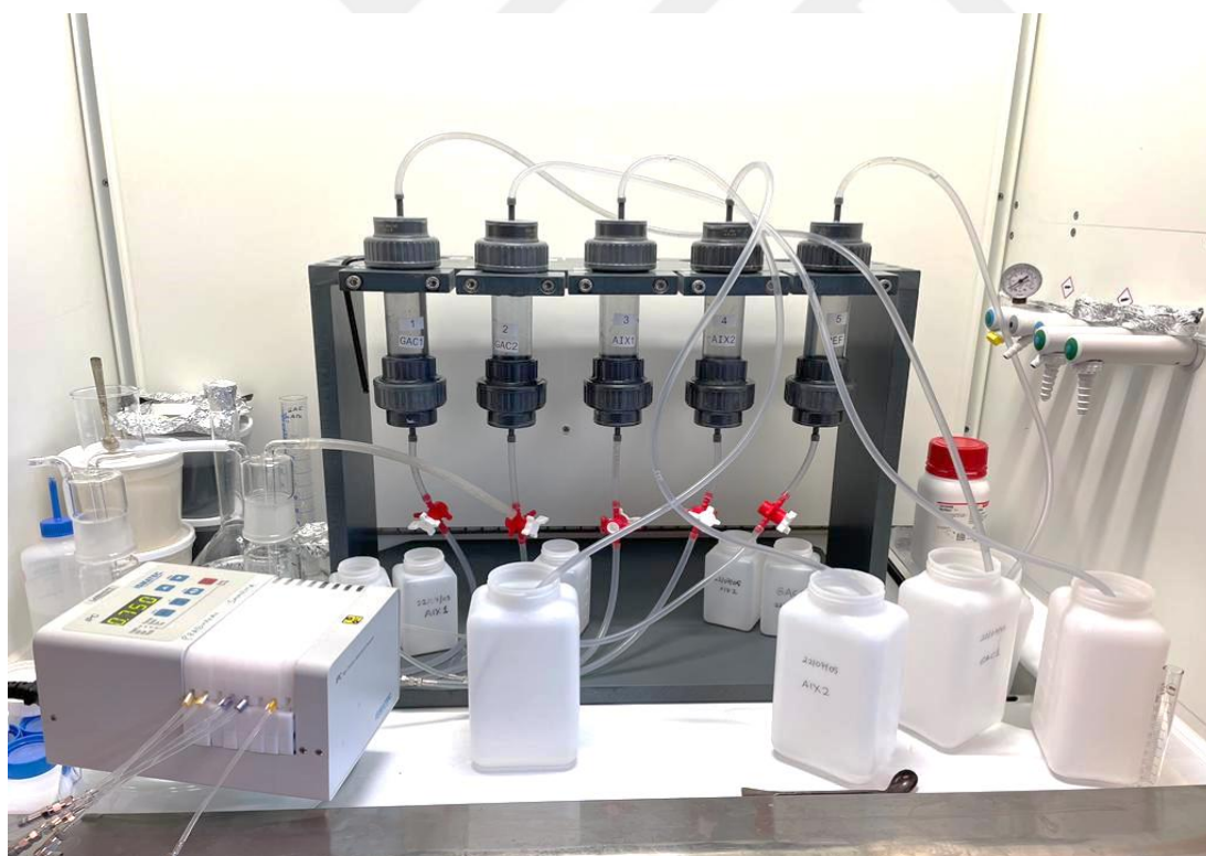
Figure 2.3 : The continuous GAC/AIX system with the necessary equipment: a multichannel peristaltic pump and plastic columns with necessary tubings.
