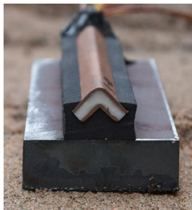
Figure 1.9 Cutting Metal Pipes with a Flexible Linear Shaped Charge [8]
