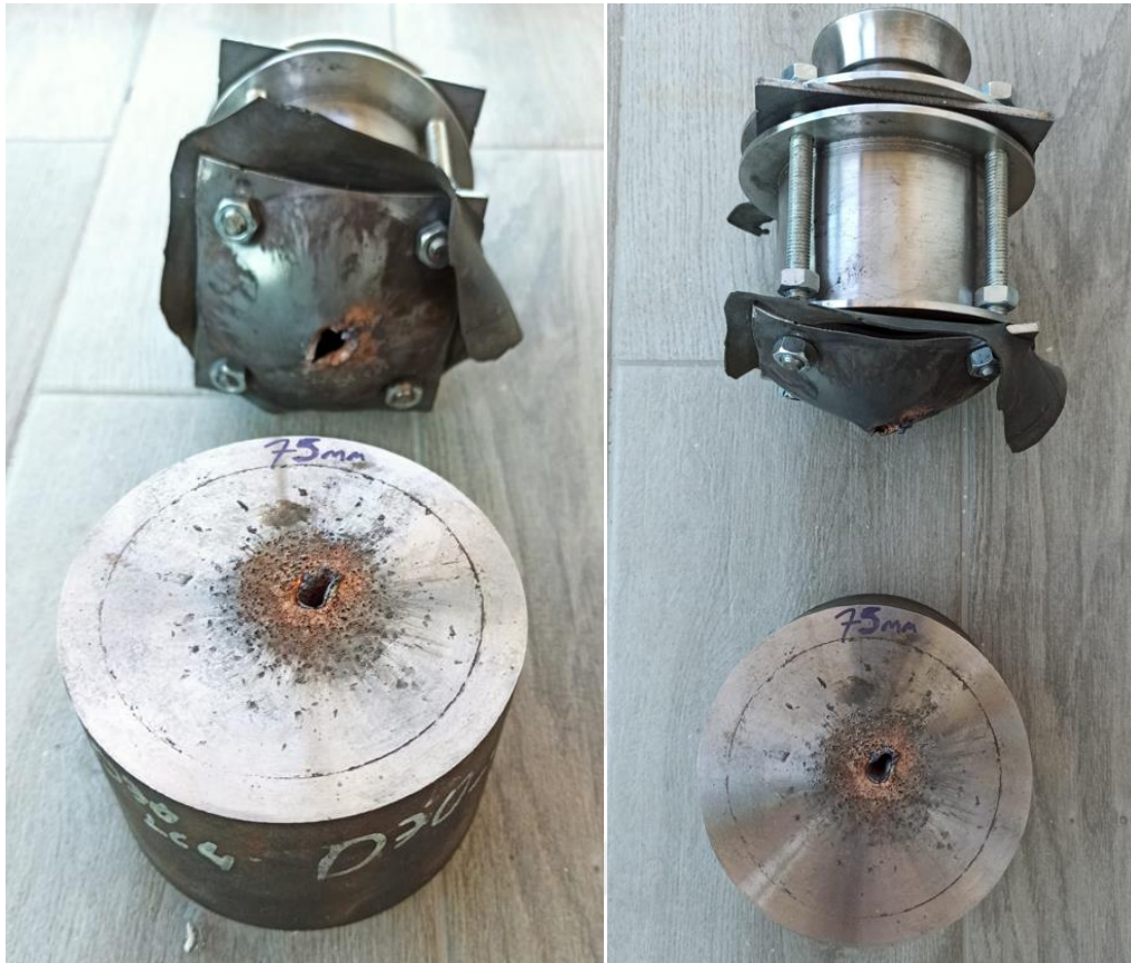
Figure A.6 Test Setup Tested with 70 mm Diameter Chamber that has 5 mm Sidewall Thickness and 64 mm Length
