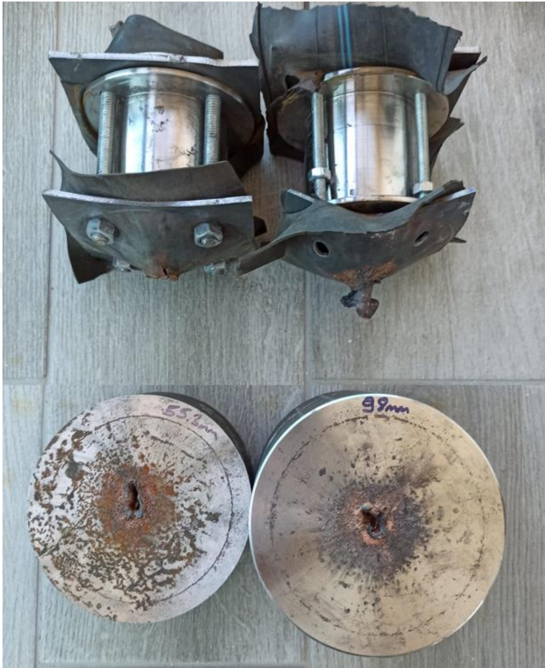
Figure A.5 Test Setups Tested with 50 mm Diameter Chambers that have 5 mm Sidewall Thickness and 64 mm Length (Two Replicates)
