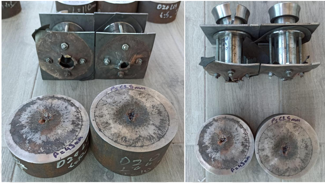
Figure C.3 Test Setups Tested with 10 mm Sidewall Thickness Chambers that have 20 mm Diameter and 64 mm Length (Two Replicates)
