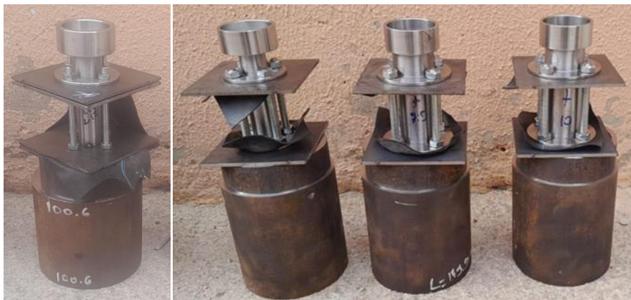
Figure 6.19 Test Setups with Different Sidewall Thickness Chambers; 1.5, 3, 7.5, and 10 mm from Left to Right, Respectively with a Standard 64 mm Length and Ø20 mm Diameter
