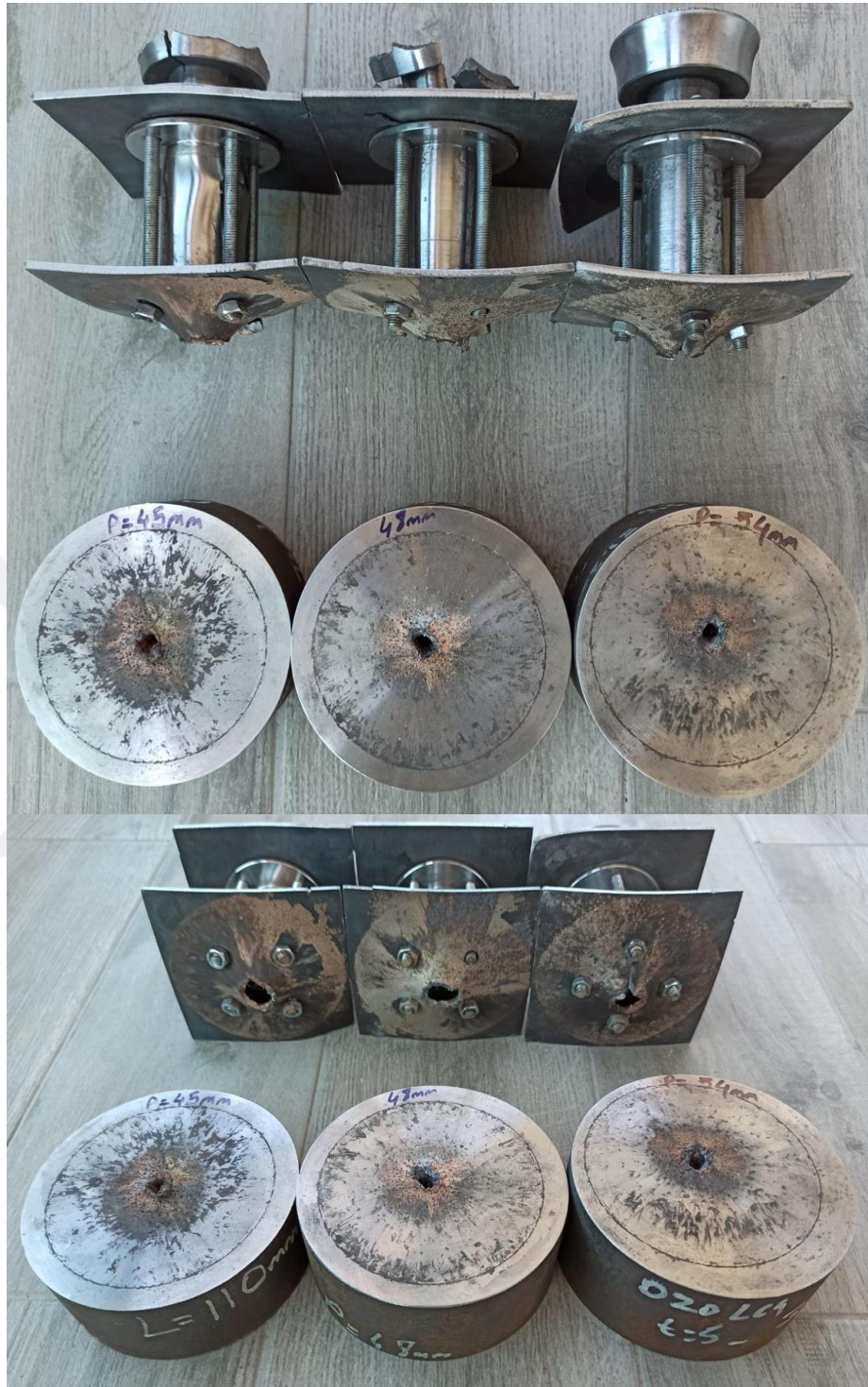
Figure A.3 Test Setups Tested with 20 mm Diameter Chambers that have 5 mm Sidewall Thickness and 64 mm Length (Three Replicates)
