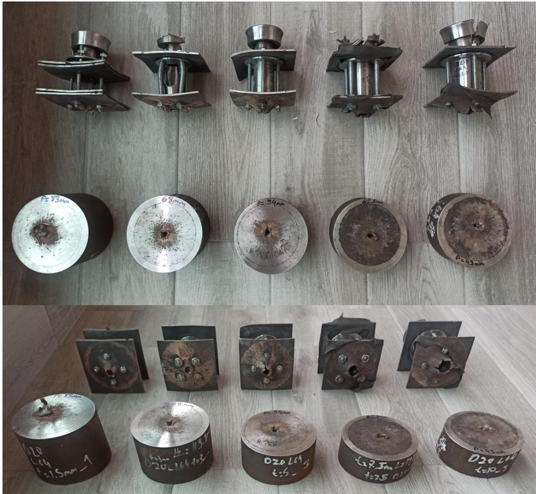
Figure 6.20 Test Results with Different Sidewall Thickness Chambers; 1.5, 3, 5, 7.5, and 10 mm, the DOP of the Witness Targets are 83, 68, 54, 42.8, and 43 mm from Left to Right, Respectively
