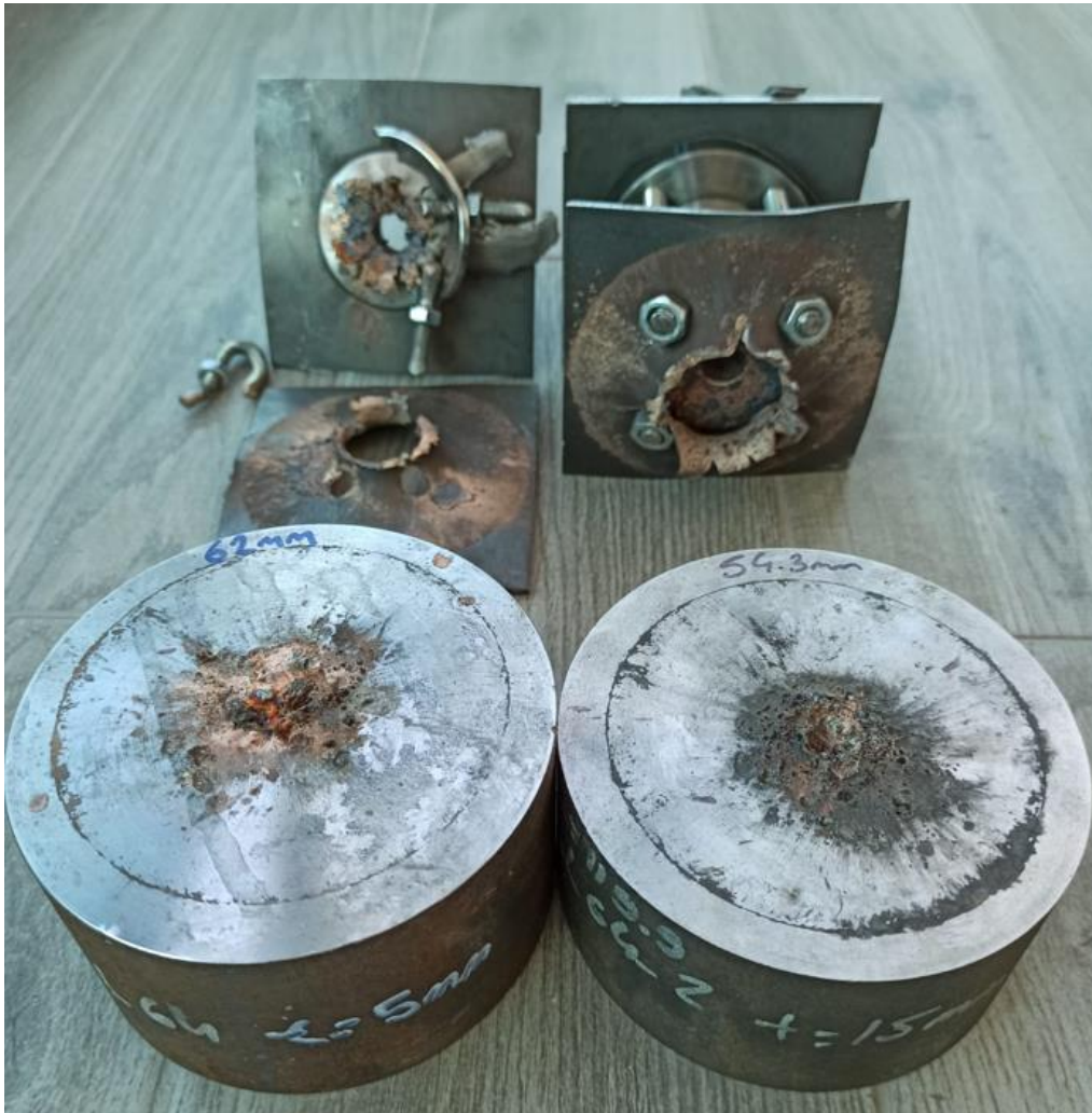
Figure A.2 Test Setups Tested with 10 mm Diameter Chambers that have 5 mm (LH Side) and 15 mm (RH Side) Sidewall Thickness and 64 mm Length
