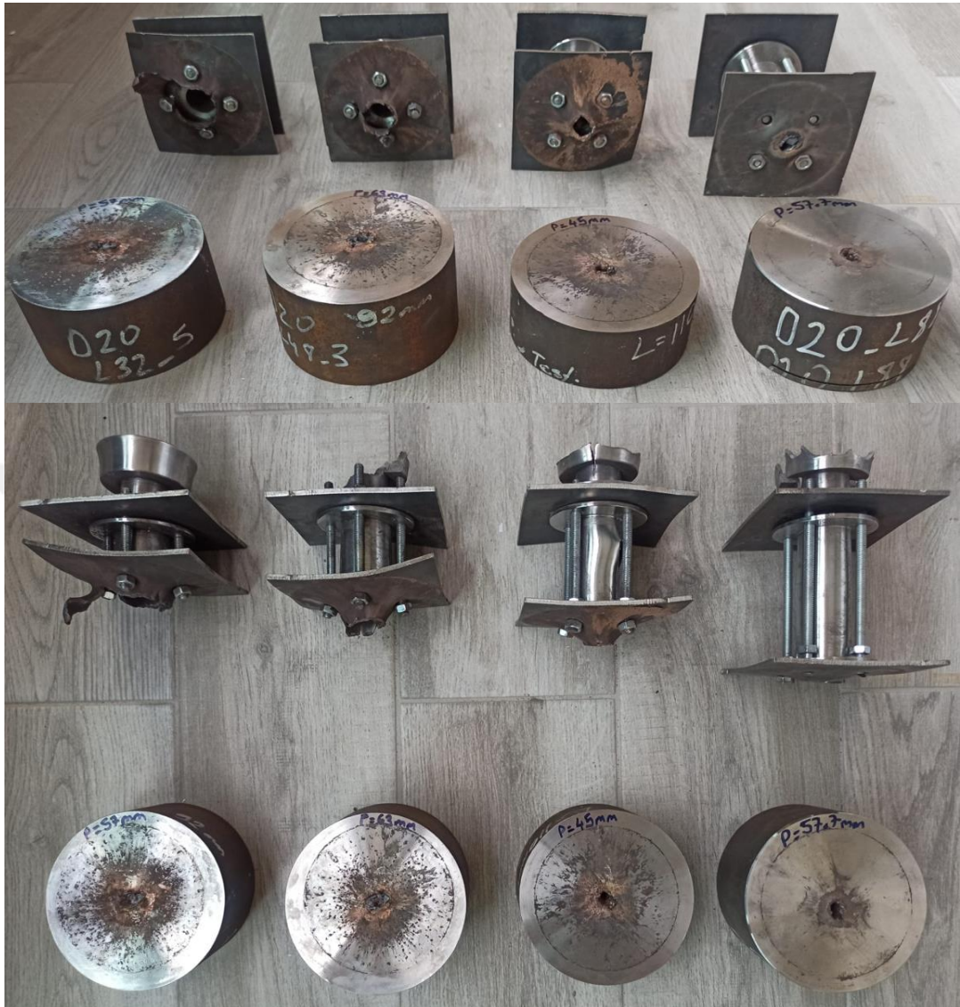
Figure 6.16 Test Results with Different Length Chambers; 32 mm, 48 mm, 64 mm and 88 mm, the DOP of the Witness Targets are 57 mm, 63 mm, 45 mm, 57,7 mm from Left to Right, Respectively
