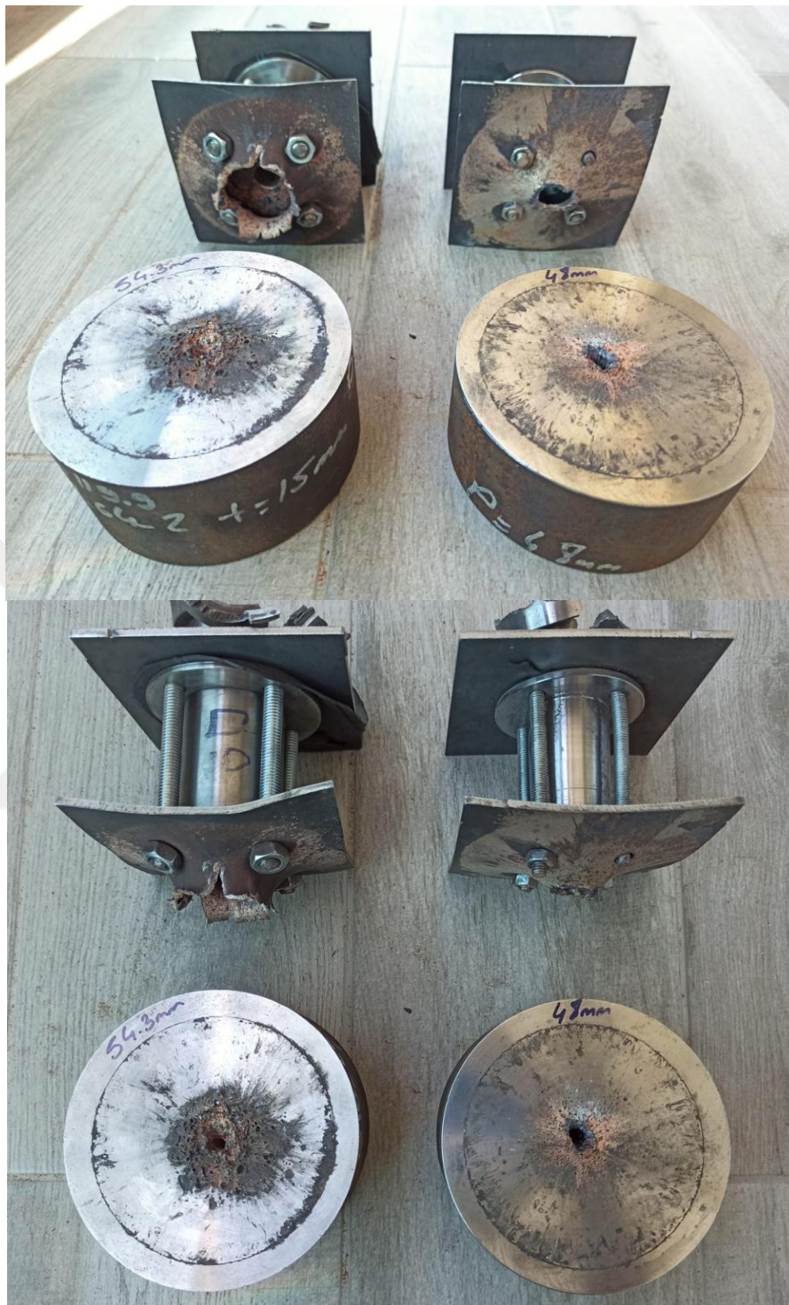
Figure 6.11 The Difference of Exit Holes between D=10 mm, t_w=15 mm (LH side Specimen in Each Picture) and D=20 mm, t_w=5 mm (RH Side Specimen in Each Picture) Diameter Chambers from Two Different Angles
