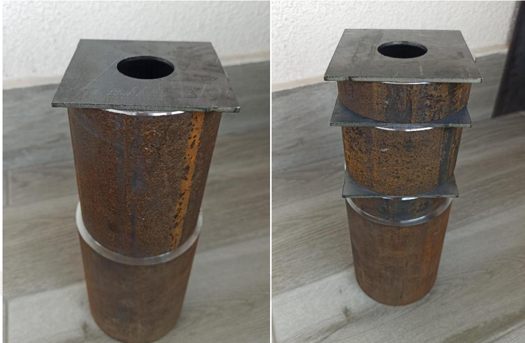
Figure 5.2 Test Setups that Represent the Cases without Chamber (LH Side), with Chamber w/o Water (RH Side)
