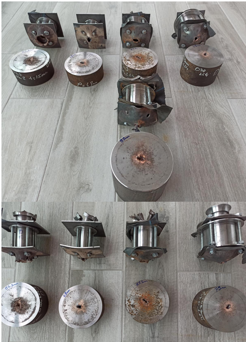
Figure 6.4 Test Results with Different Diameters; \text{\O}10 mm (15 mm sidewall thickness), 20 mm, 50 mm and 70 mm, the DOP of the Witness Targets (the Height of the Machined Target from the Bottom) are 55 mm, 48 mm, 55.3 mm, 75 mm from Left to Right, Respectively
