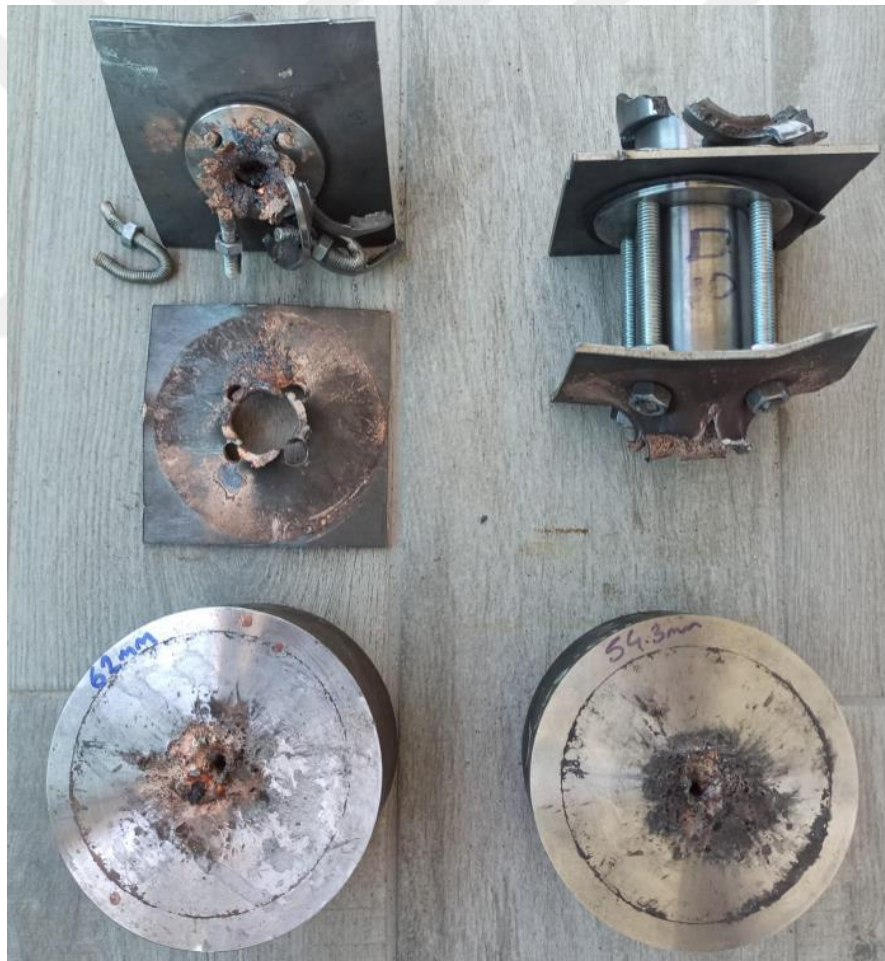
Figure 6.6 Test Specimens and Witness Plates for D=10 mm Chamber Diameter, t_w=5 mm Sidewall Thickness (LH Side), t_w=15 mm (RH Side)
