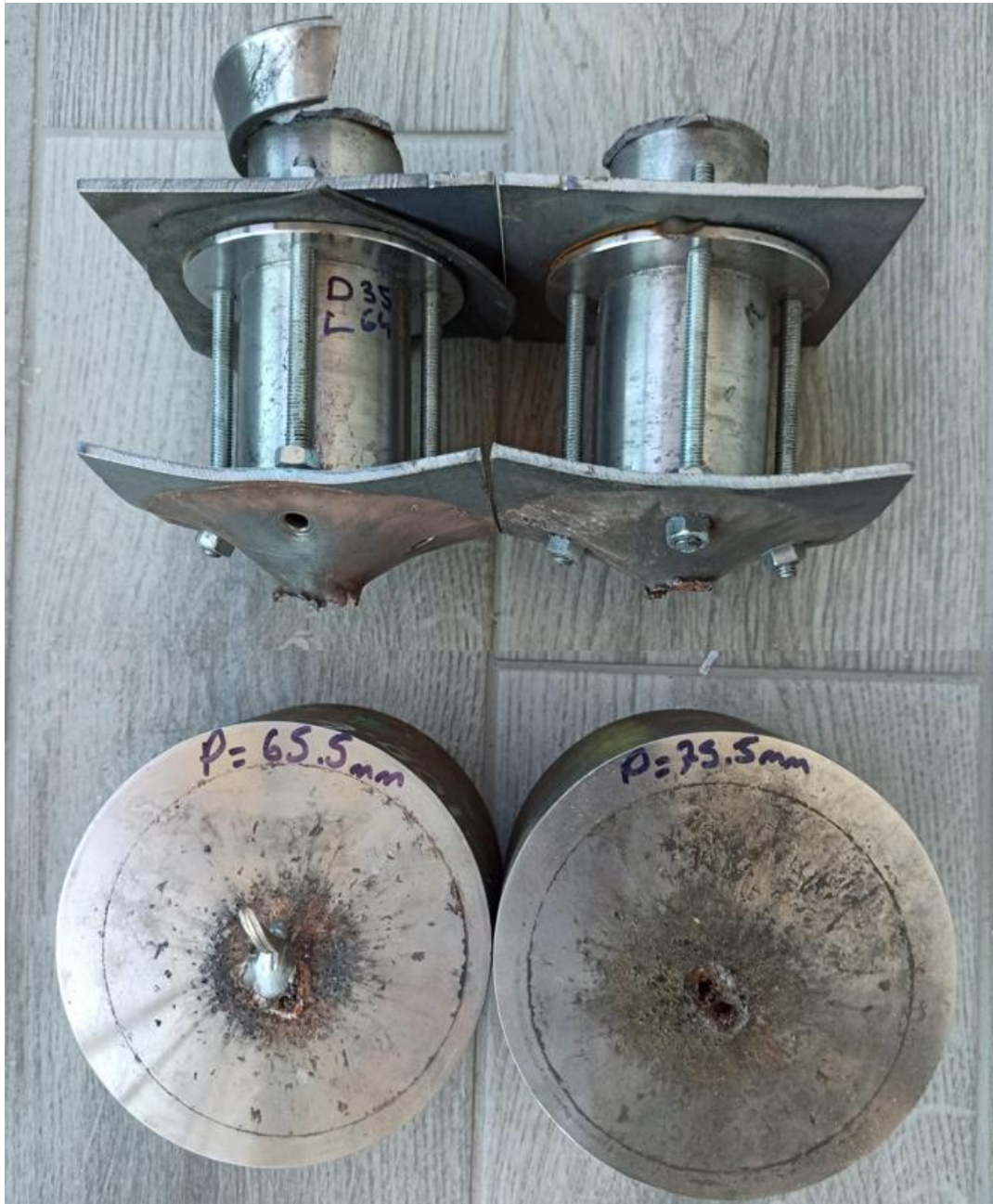
Figure A.4 Test Setups Tested with 35 mm Diameter Chambers that have 5 mm Sidewall Thickness and 64 mm Length (Two Replicates)
