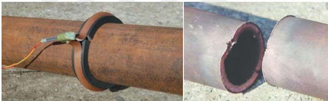
Figure 1.9 Cutting Metal Pipes with a Flexible Linear Shaped Charge [8]
