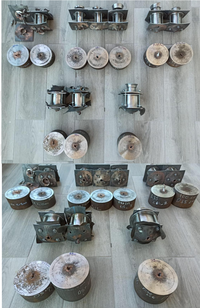
Figure A.1 Test Setups Tested with Chambers that have 10, 20, 35 (Above), 50, and 75 mm (Below) Diameter and 64 mm Length
