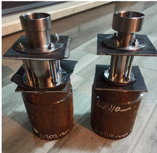
Figure 5.3 Test Setups with \text{\O}50 mm Diameter and 64 mm Length Chamber (LH Side), with \text{\O}20 mm Diameter and 64 mm Length Chamber (RH Side)
