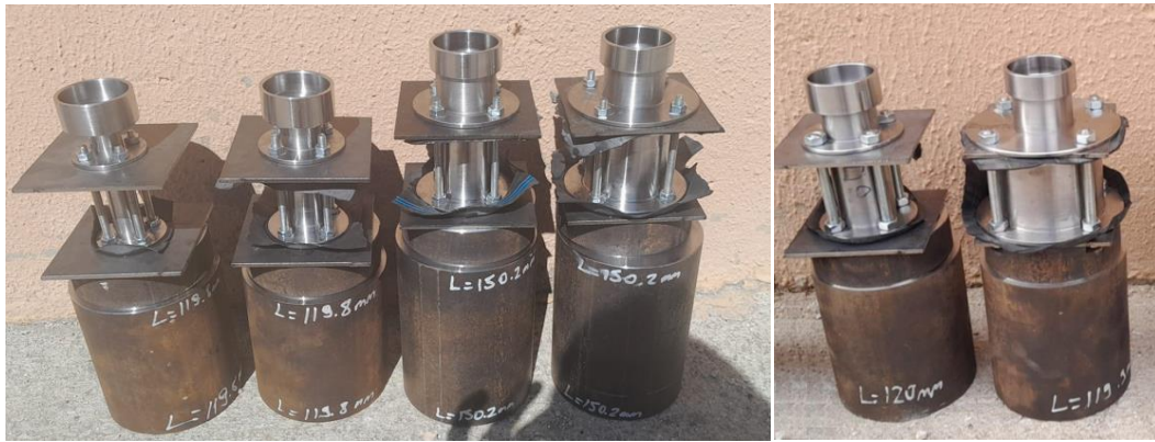
Figure 6.2 Test Setups with \text{Ø}10 , 20, 35, 50 mm Diameter Chambers (LH Side Picture), \text{Ø}10 Diameter, 15 mm Sidewall Chamber and a \text{Ø}70 mm Diameter Chamber (RH Side Picture) from Left to Right, Respectively with a Standard 5 mm Sidewall Thickness (Except Mentioned) and 64 mm Length
