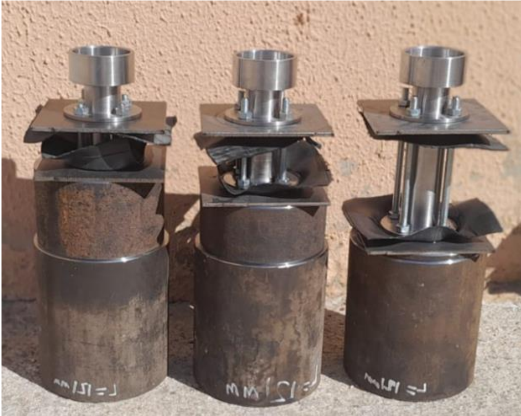
Figure 6.15 Test Setups with Different Length Chambers; 32 mm, 48 mm and 88 mm from Left to Right, Respectively with a Standard 5 mm Sidewall Thickness and \text{Ø}20 mm Diameter
