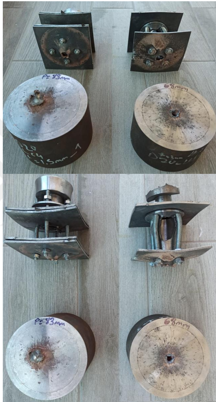
Figure C.1 Test Setups Tested with 1.5 (LH Side in Each Picture) and 3 mm (RH Side in Each Picture) Sidewall Thickness Chambers that have 20 mm Diameter and 64 mm Length
