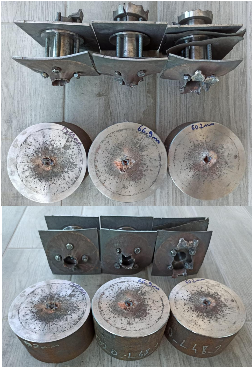
Figure B.3 Test Setups Tested with 48 mm Long Chambers that have 5 mm Sidewall Thickness and 20 mm Diameter (Three Replicates)
