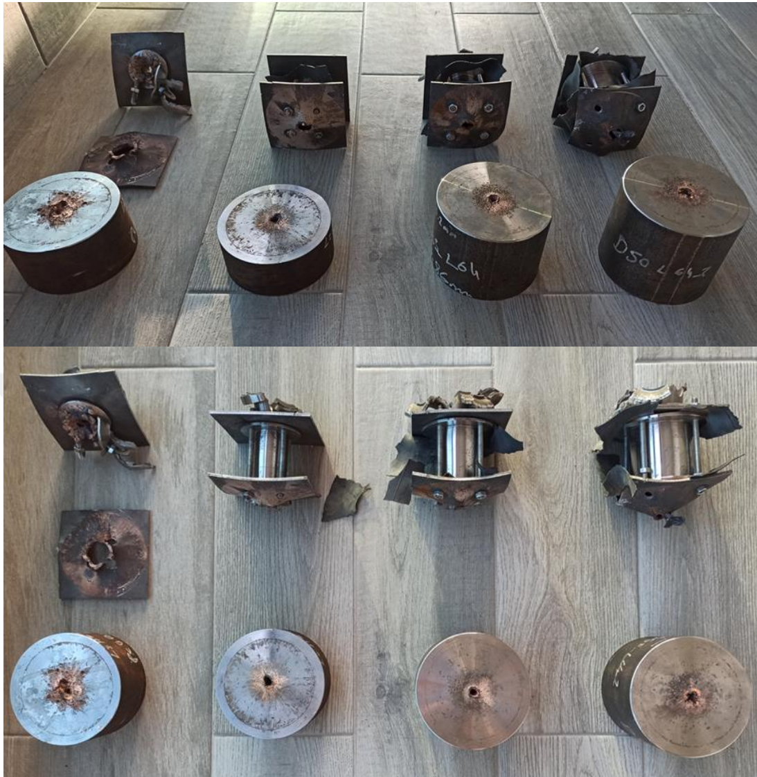
Figure 6.3 Test Results with Different Diameters; \text{\O}10 mm, 20 mm, 35 mm and 50 mm, the DOP of the Witness Targets (the Height of the Machined Targets from the Bottom) are 62 mm, 48 mm, 75.5 mm, 98 mm from Left to Right, Respectively
