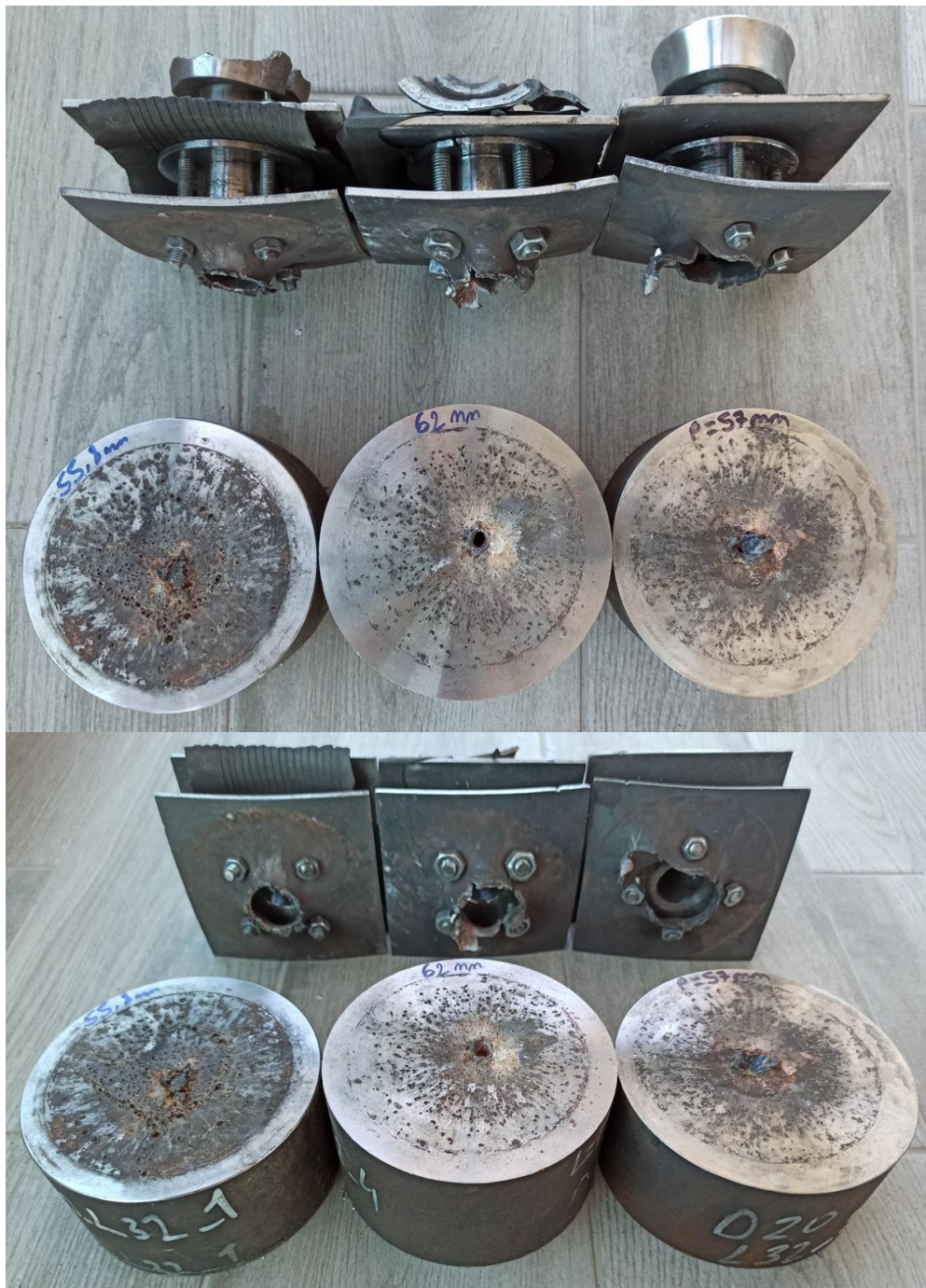
Figure B.2 Test Setups Tested with 32 mm Long Chambers that have 5 mm Sidewall Thickness and 20 mm Diameter (Three Replicates)
