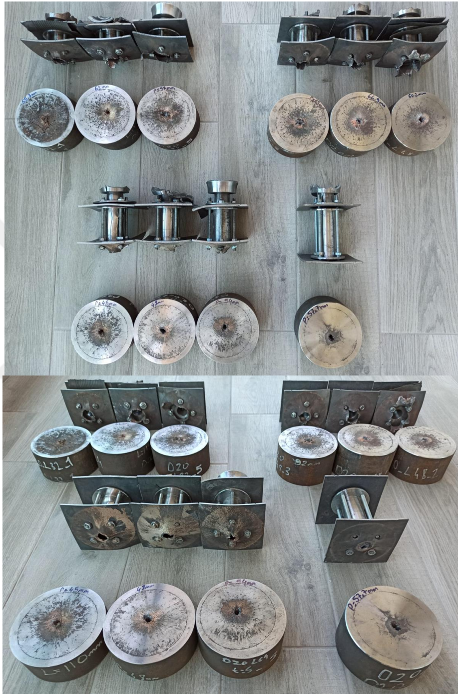
Figure B.1 Test Setups Tested with 32, 48 (Above), 64, and 88 mm (Below) Long Chambers that have 20 mm Diameter and 5 mm Sidewall Thickness
