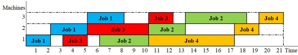
Figure 2.1. An example for NWPFSF with 4 jobs on 3 machines
