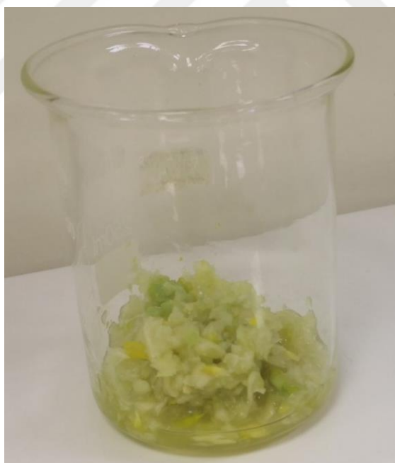
Figure 3.1 200 grams of garlic cloves that had been peeled and crushed in a homogenizer using cold distilled water
