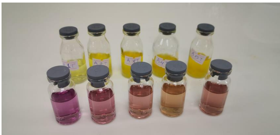
Figure 3.13 The yellowish reduced form the stable violet DPPH radical of the Ajoene extract samples
