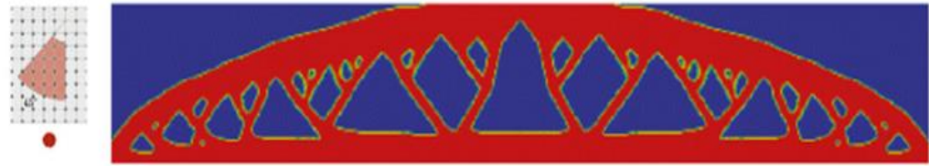
b Solution with minimum self-supporting angle of 45 degrees,, f = 116.11 , f_{\eta=0} = 108.38 .
