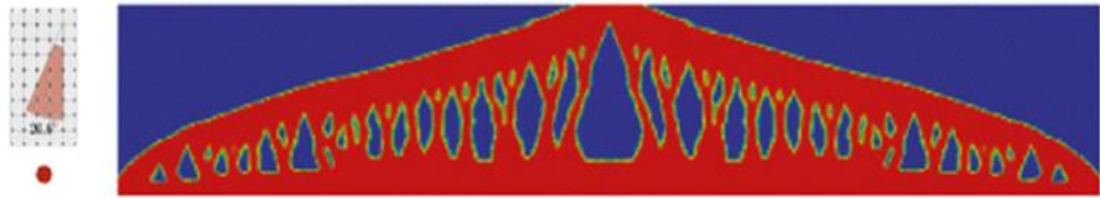
c Solution with minimum self-supporting angle of 63.4 degrees,, f = 174.69 , f_{\eta=0} = 158.95 .
