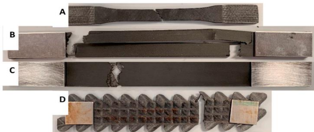
Figure 6: fracture modes observed during tensile testing[40].
