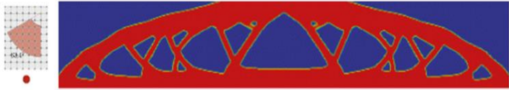
a Solution with minimum self-supporting angle of 26.6 degrees, f = 109.53 , f_{\eta=0} = 103.42 .
