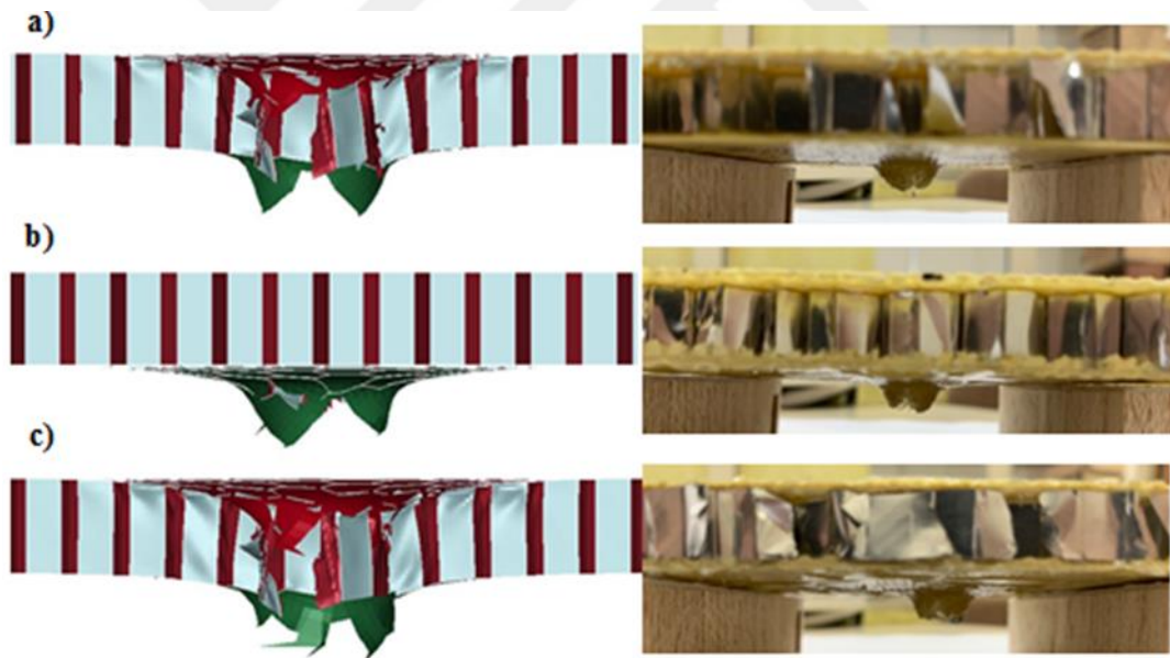
Figure 5.11 Comparative damage models of HC-core sandwich composites with Kevlar/epoxy in configurations: a) neat, b) 0.5%, and c) 1% nano clay by weight, derived from QS-PS tests through experimental and simulation results at 1.25 mm/min
