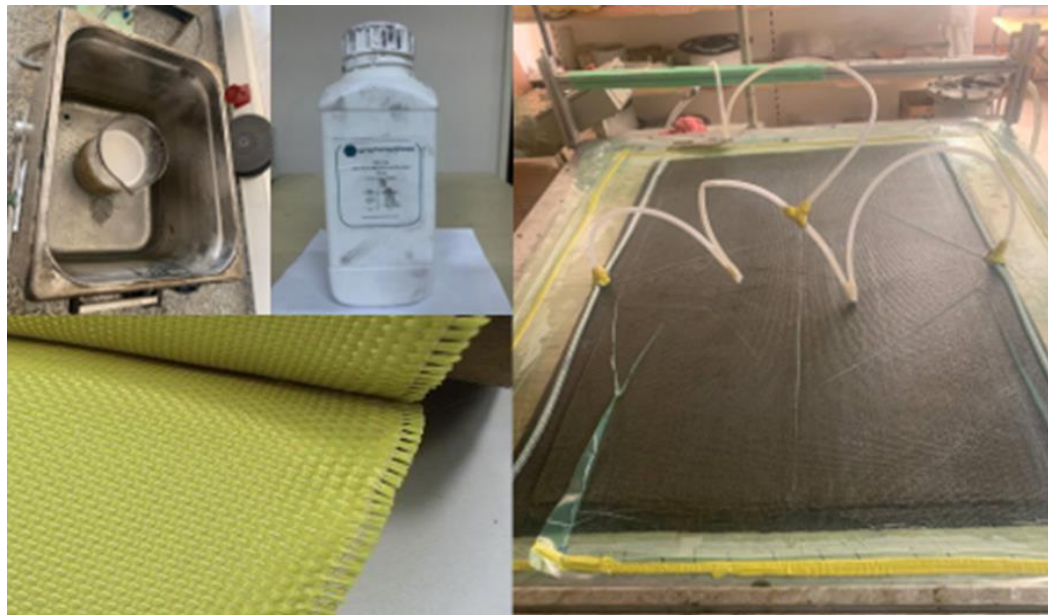
Figure 3.2 Fabrication process of Kevlar/epoxy plates with varying nanoclay concentrations (neat, 0.5%, and 1% by weight)
