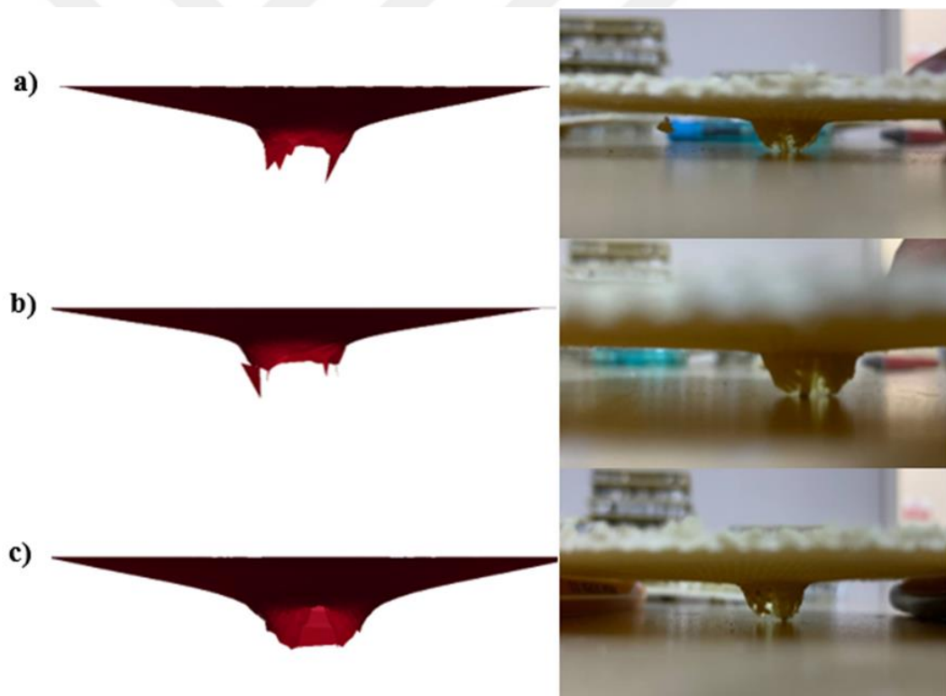
Figure 5.20 Comparison of damage models for Kevlar/epoxy composites for a) neat, b) 0.5%, and c) 1% nano clay by weight from QS-PS tests: experimental vs. simulation at 25 mm/min
