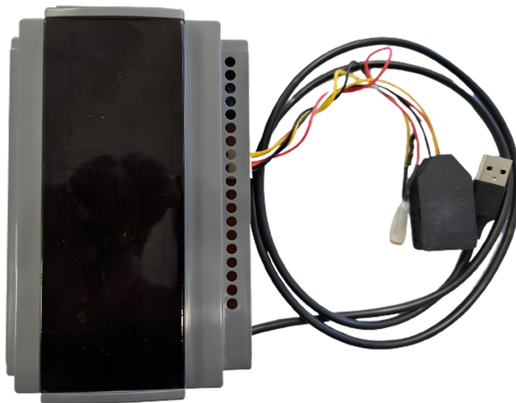
Figure 3.6. Completed version of the remote monitoring hardware.
