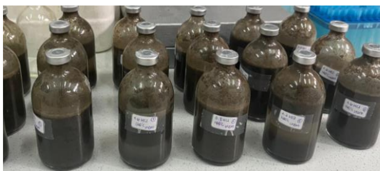
Figure 3.5 : Anaerobic digestion setup.
