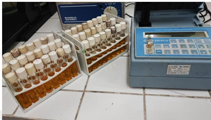
Figure 3.7 : sCOD measurement with HACH DR/2010 portable datalogging spectrophotometer at 600 nm.
