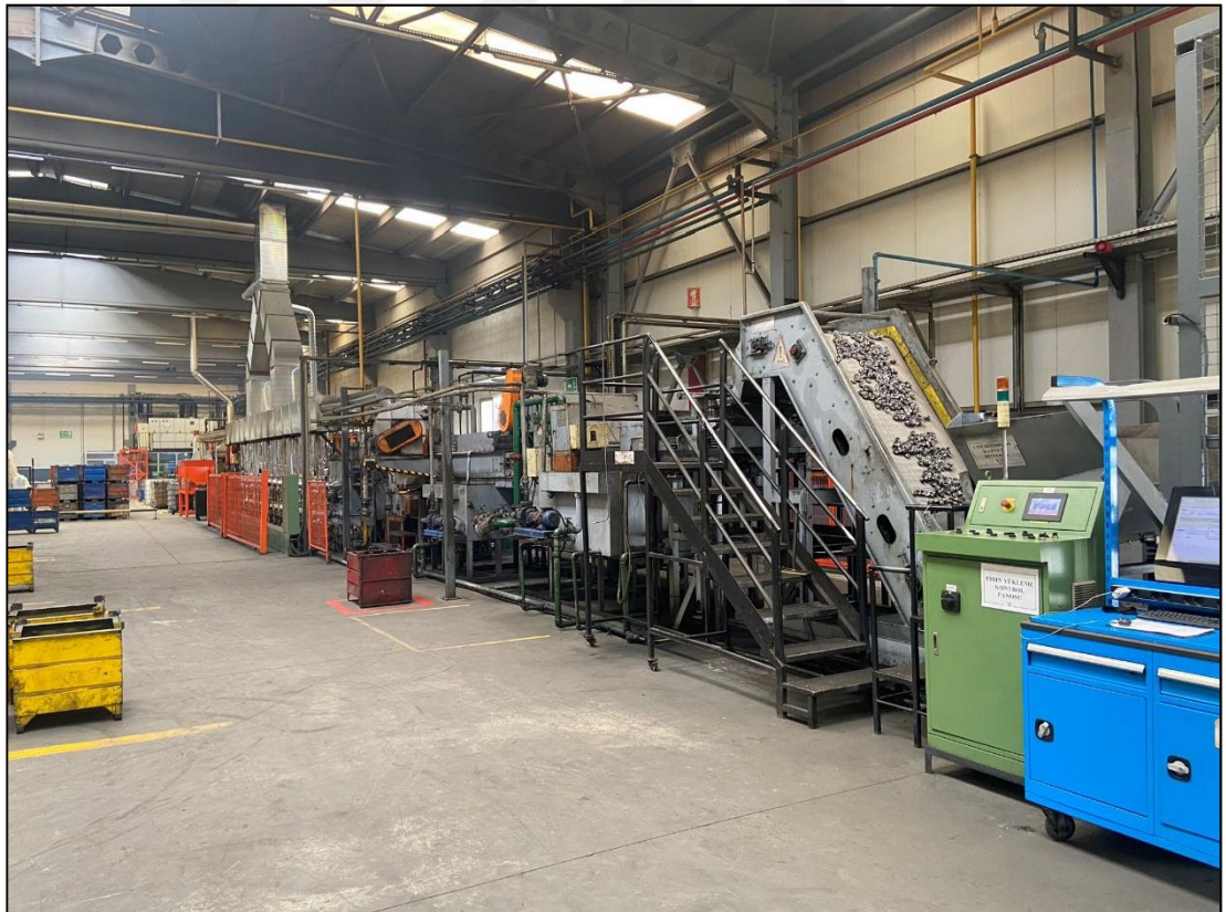
Figure 3.10 Heat treatment line
