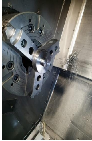
Photo 3.12 Pictures of the production of the modified MB pump on a 4-axis CNC machine (Personal archive,2023)
