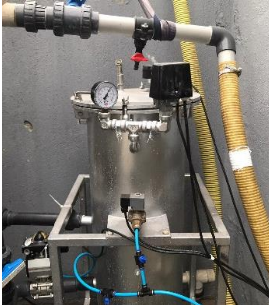
Photo 3.2 The pressure tank of CP-DAF System used in the field studies (Personal archive, 2022)
