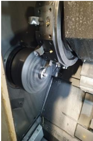
Photo 3.12 Pictures of the production of the modified MB pump on a 4-axis CNC machine (Personal archive,2023)
