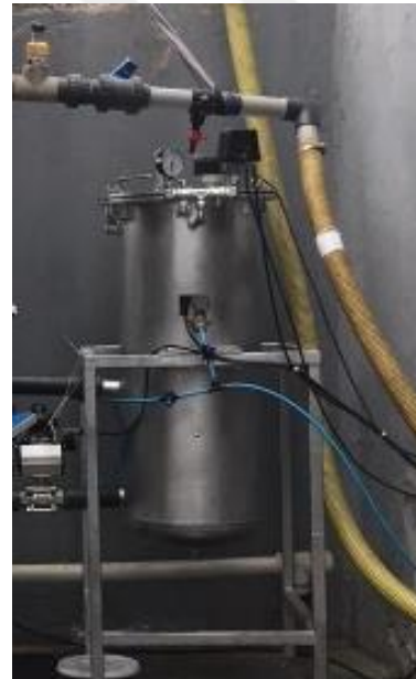
Photo 3.3 The pressure tank of CP-DAF System used in the field studies, (Personal archive, 2022)
