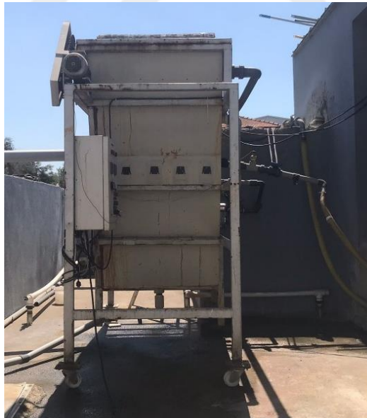
Photo 3.4 Images of MB-DAF-1 System on Pilot DAF used in Field Studies (Personal archive, 2022)
