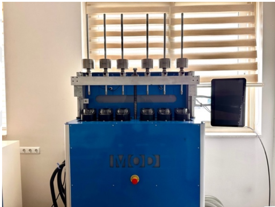
Figure 3.40. Chewing Simulator (MOD Chewing Simulator, Esetron; MOD Dental, Ankara, Turkey)
