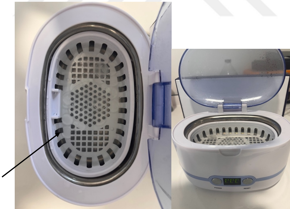
Figure 3.26. and Figure 3.27. Samples cleaned in distilled water for 10 minutes with ultrasonic cleaner (AS 8772 Ultrasonic Cleaner, General Home Orsay Ltd. Şti., İstanbul, Turkey)
