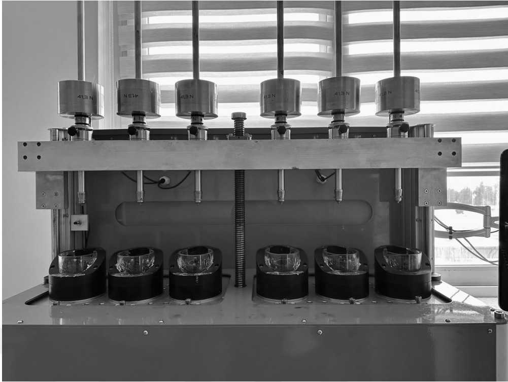
Figure 2.10. Chewing Simulator (MOD Chewing Simulator, Esetron; MOD Dental, Ankara, Turkey)
