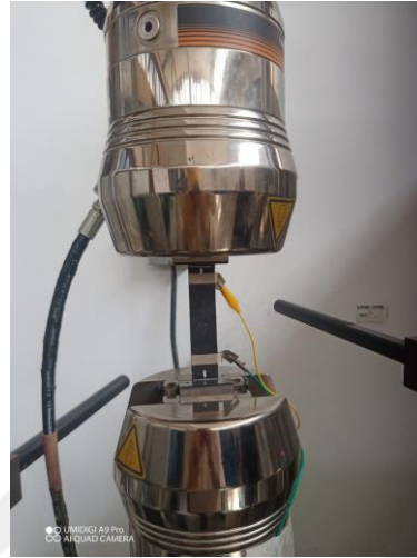
Figure 3.5. The test setup for measuring electrical resistance change during fatigue test
