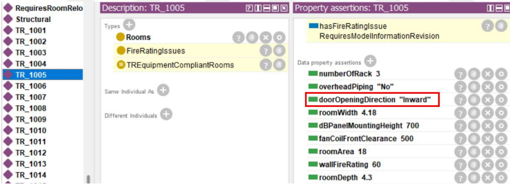
Figure 4.20 Non-compliance of TR_1005.
