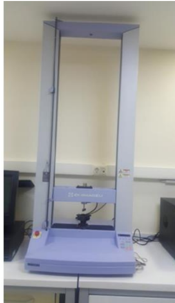
Resim 3.9. Evrensel Test Cihazı (Shimadzu Autograph AGS-J Series, Kyoto, Japan)
