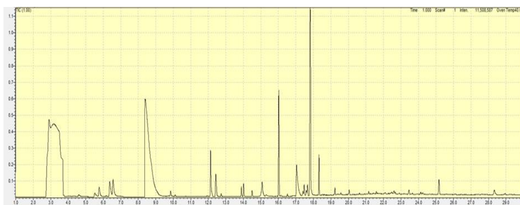
Figure 4.16 The sample chromatogram of SPME-GC-MS analysis of EBC for lung cancer patient
