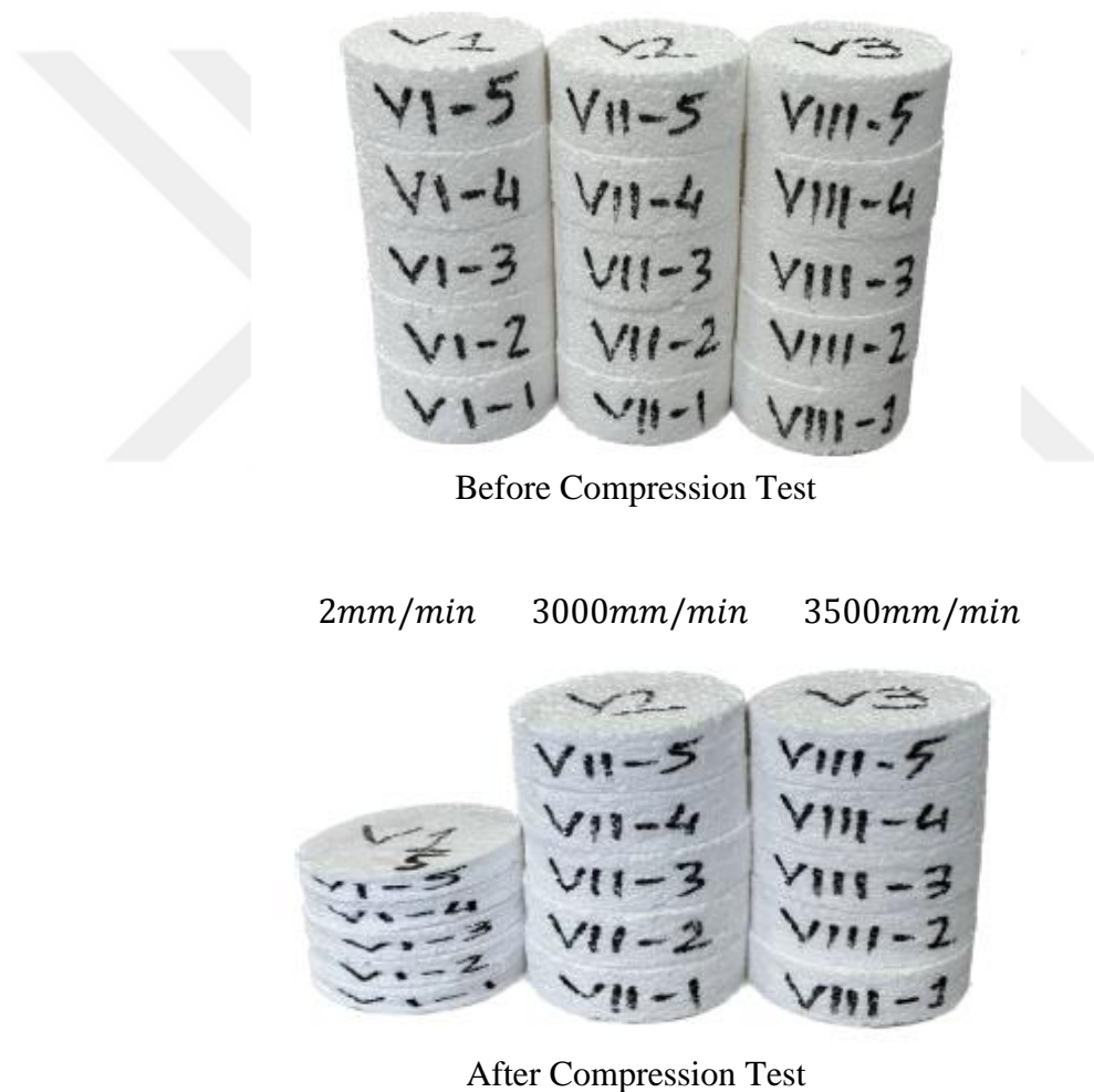
Figure 4.2 Foam specimens before and after the uniaxial compression test
