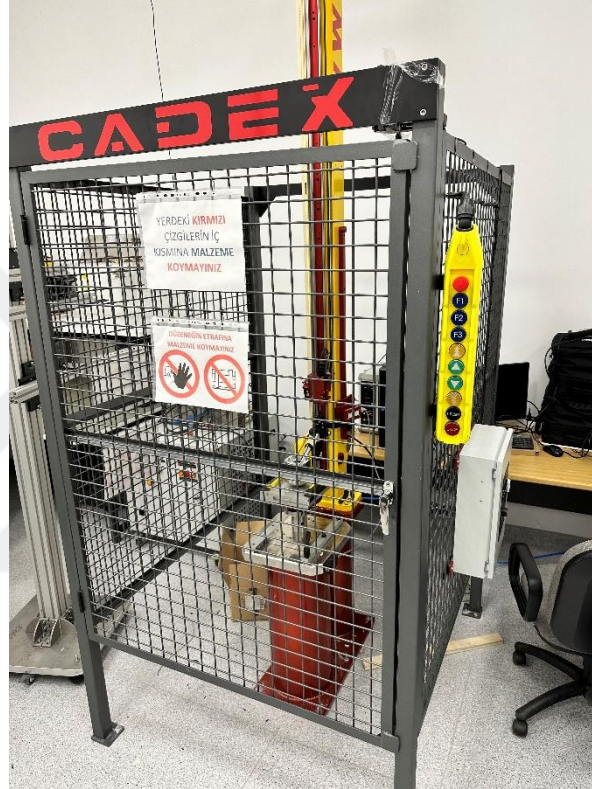
Figure 5.1 CADEX Monorail Impact Setup
