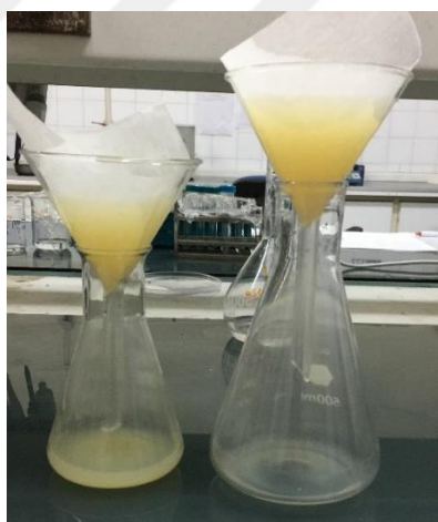
Figure 6.1 : Filtration step before microfluidization of liposomes.
