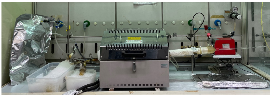
Figure 2.2: Fixed-bed furnace apparatus during a pyrolysis test.
