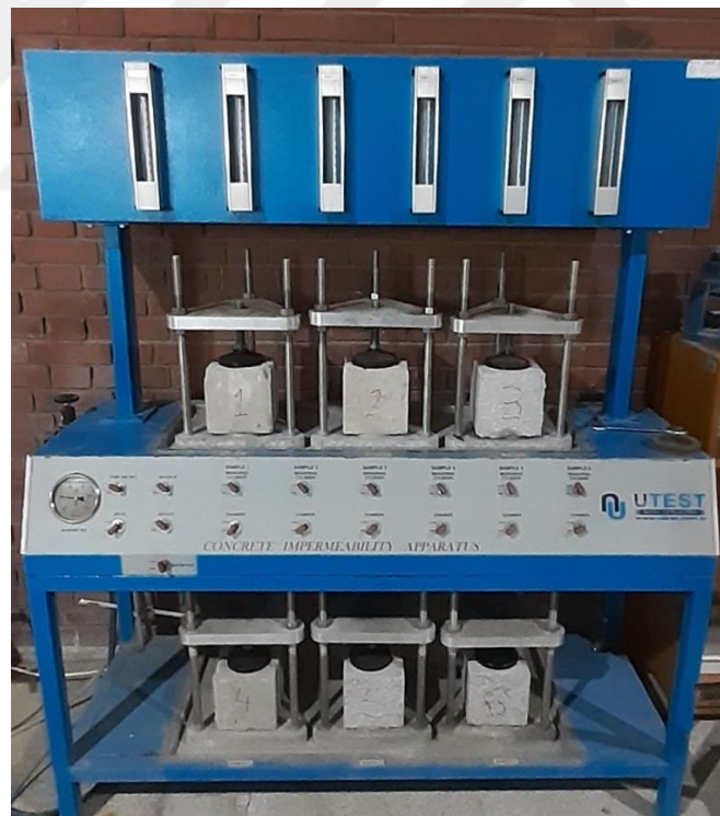
Figure 4. 1. Pressurized water experiment setup
