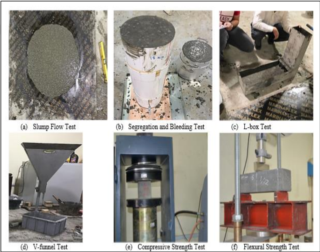
Figure 2.6: Fresh and hardened concrete tests [47].
