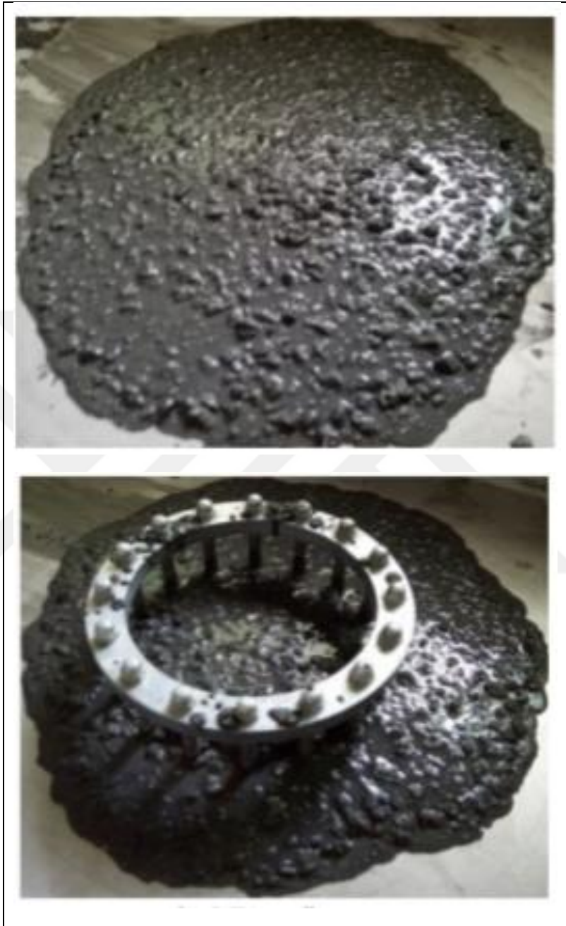
Figure 2.1: Configuration of the slump flow and ring flow testing process [41].
