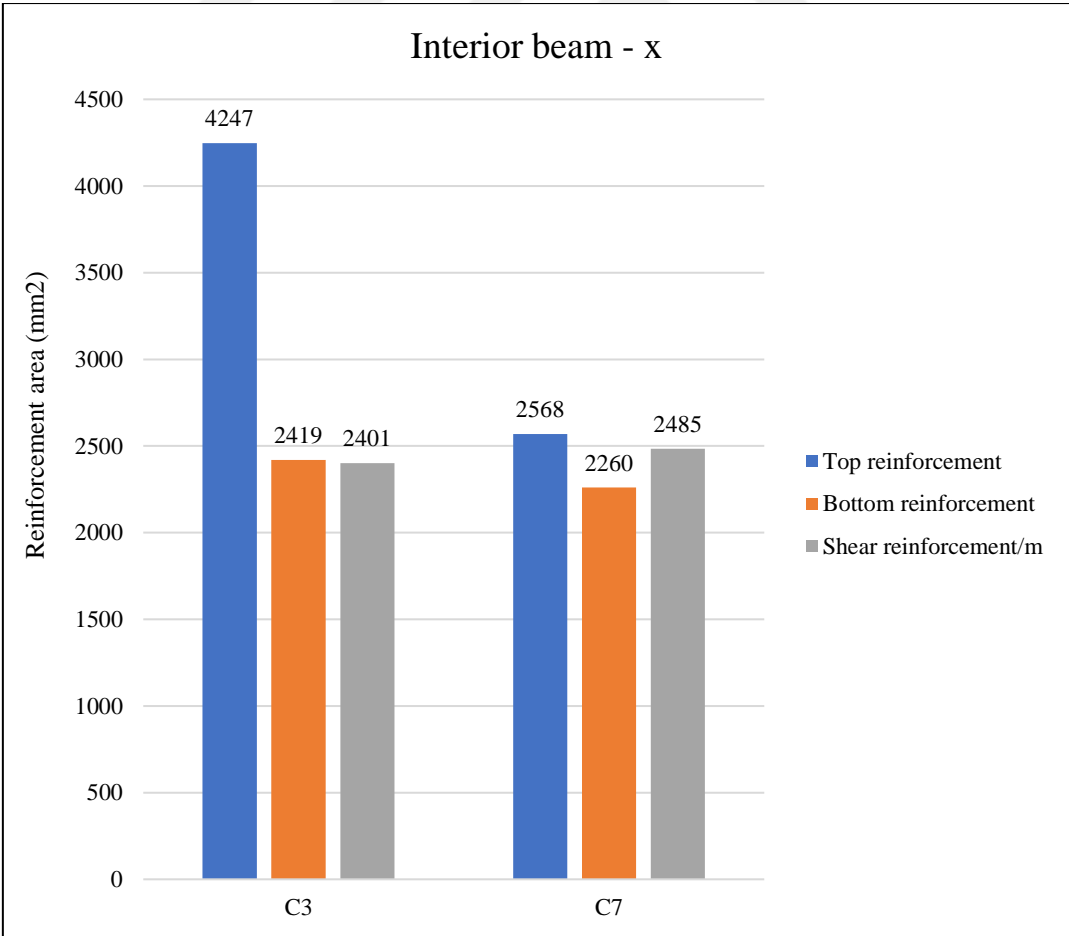
Figure 4.33: Interior beam-x reinforcement for Cases C3 and C7.
