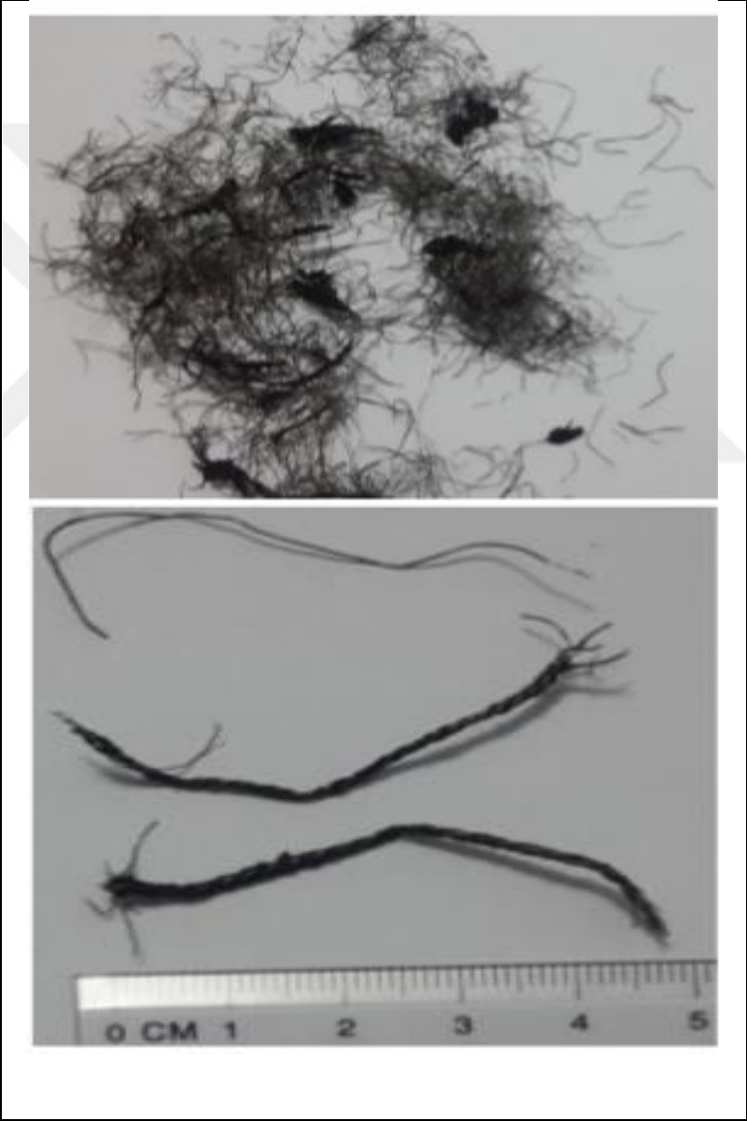
Figure 2.4: A Configuration of the recycled steel fiber [46].
