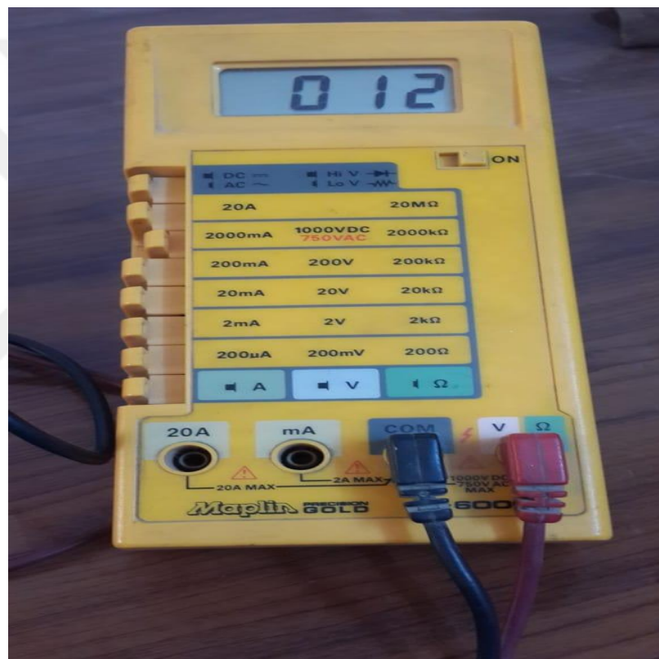
Figure 3.9: Maplin Digital multimeter for voltage and current measurements
