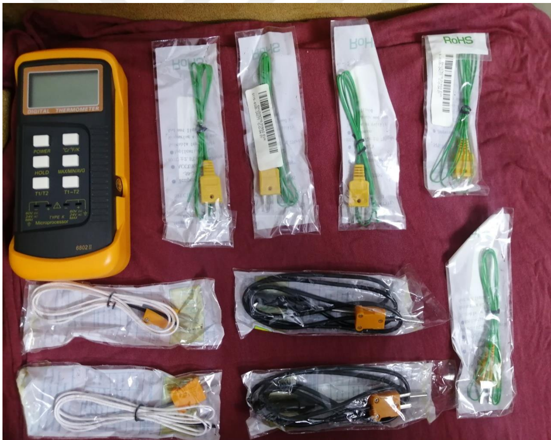
Figure 3.7: Digital Thermometer for temperature measurements.
