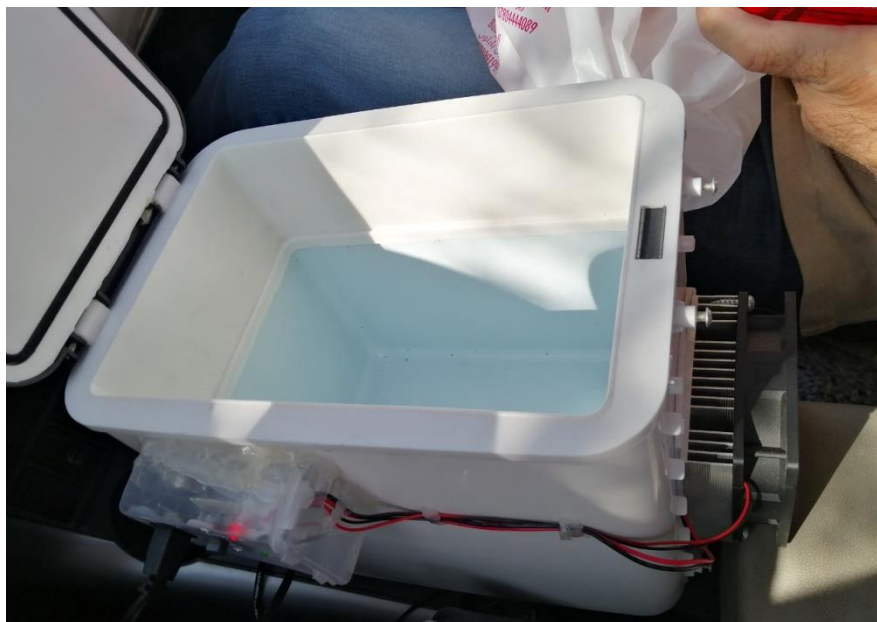
Figure 3.13: Fixing the control box on the insulating box.
