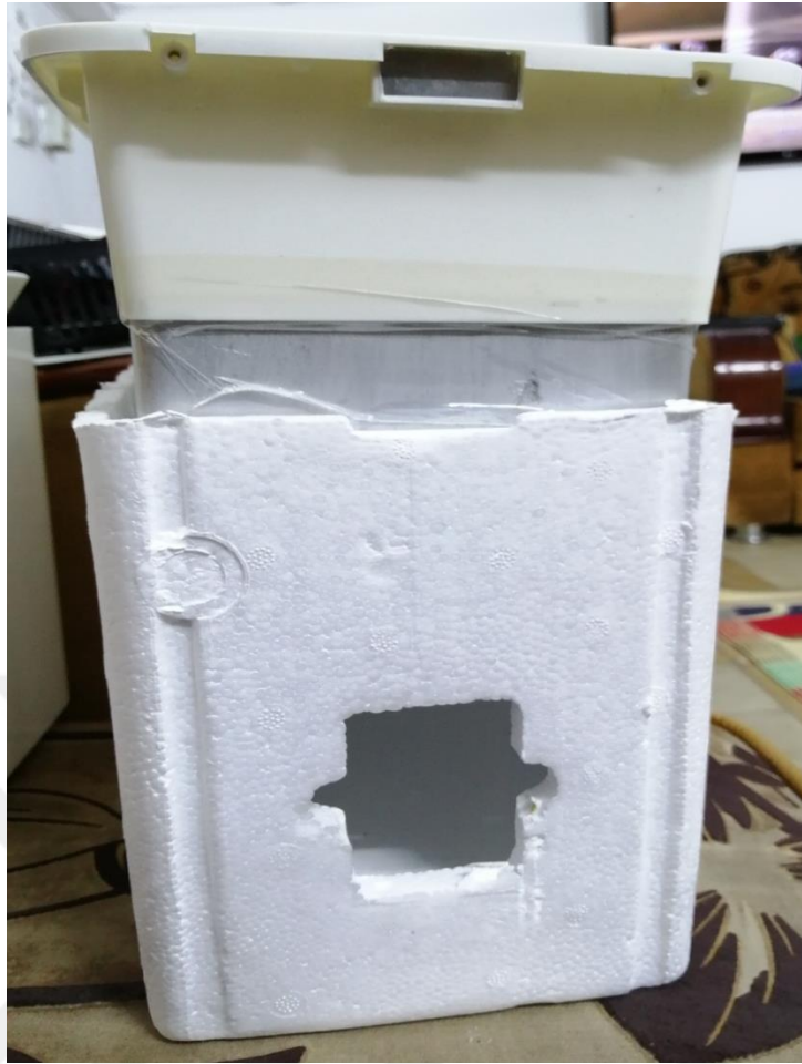
Figure 3.11: Insertion of the thermocol box between the inner and outer plastic walls of the box.
