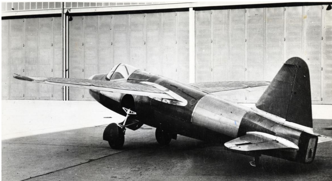
Figure 2: The first aircraft flying with turbojet engine by Von Ohain [4]
