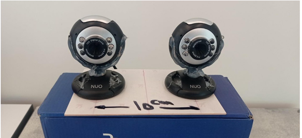
Figure 4.2: 2 NUO cameras with focal length of 3.85mm megapixel 10x Digital zoom. Mounted on a flat prime base 10cm apart.
