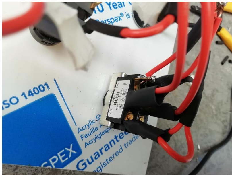
Figure 28: Replacing the Switches
