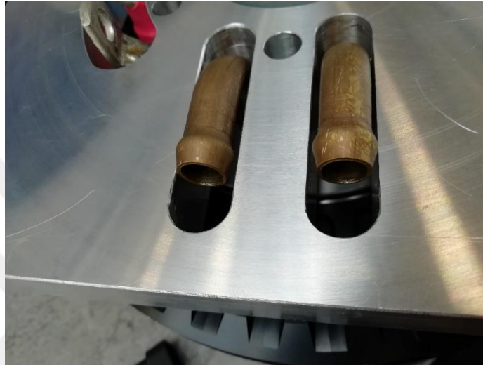
Figure 24: EMRAX 208 Cooling Pipe Protrusions on Motor Mount Plate
