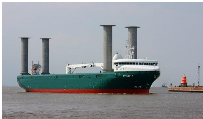
Figure 4.6 : “E-Ship 1” with 4 Flettner rotors.
