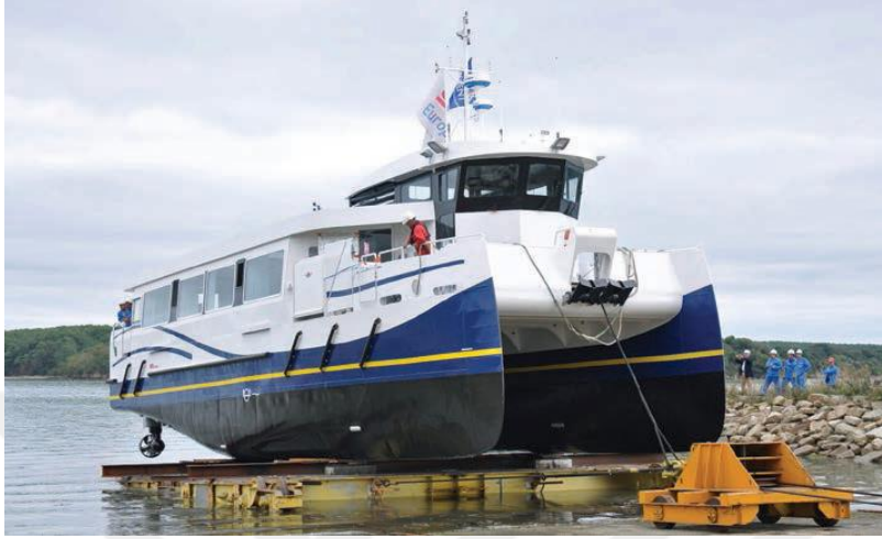
Figure 4.4 : “Ar Vag Tredan” supercapacitor driven ferry.
