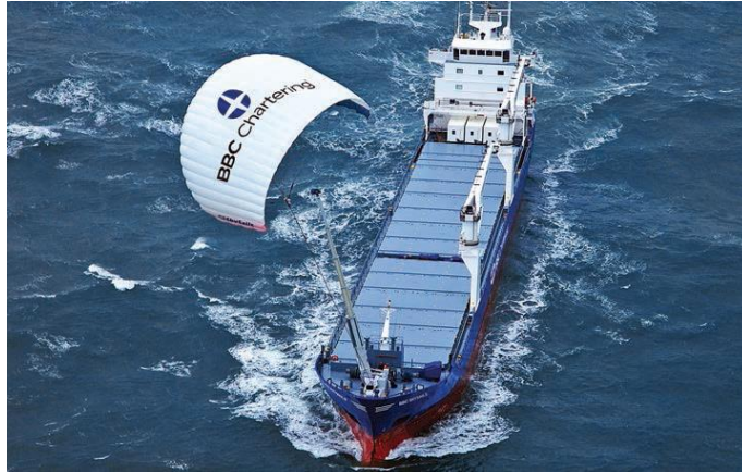
Figure 4.7 : Kite assists to propulsion.
