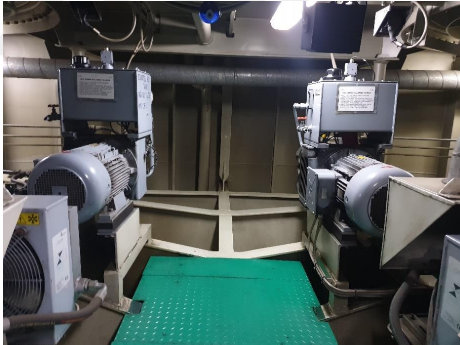
Figure 1.3: Electric motors to drive the propeller of the case ship.
