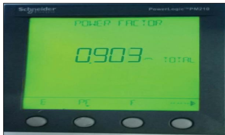
Figure 2.2: Corrected power-factor value after applying IPFC [4]
