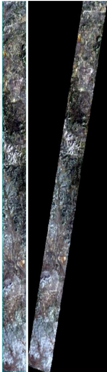
Figure 6.14 Image before (left) and after (right) geo-registration
