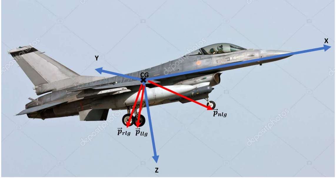
Figure 2.7 Position vectors of F-16 landing gears [49]
