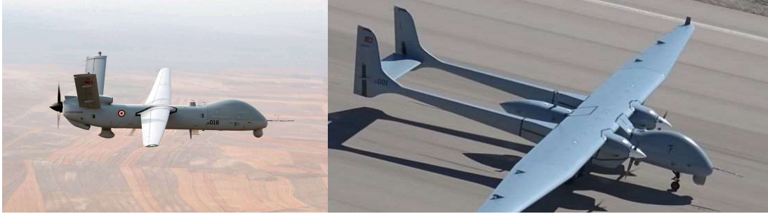
Figure 1.5 a. TAI Anka drone [4] that use an autoland system, Figure 1.5 b. TAI Aksungur drone [5] also uses an autoland system.
