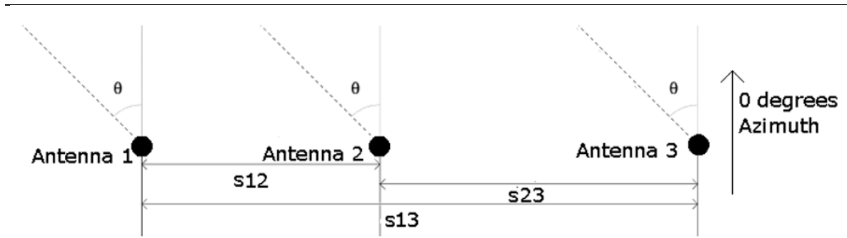
Figure 4.8: Three-antennas phase interferometry systems geometry [6]
