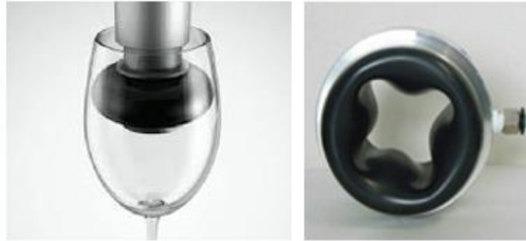
Figure 16. Inside (left) and outside (right) type bellow grippers
