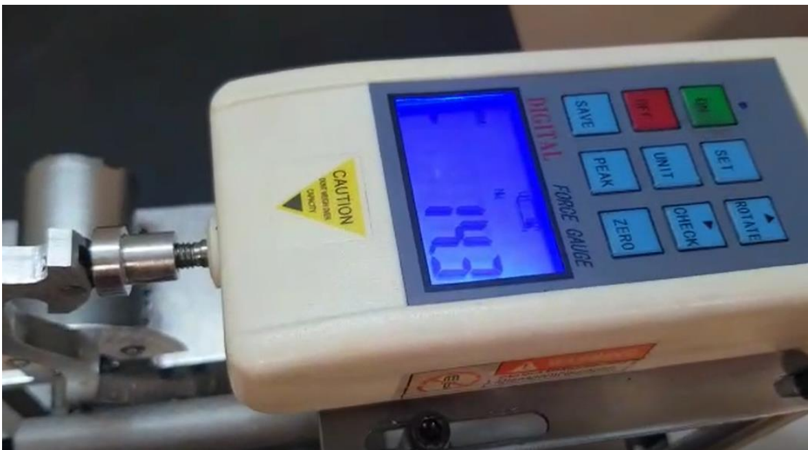
Figure 83. Measurement at \alpha_F = 102^\circ with spring removed
