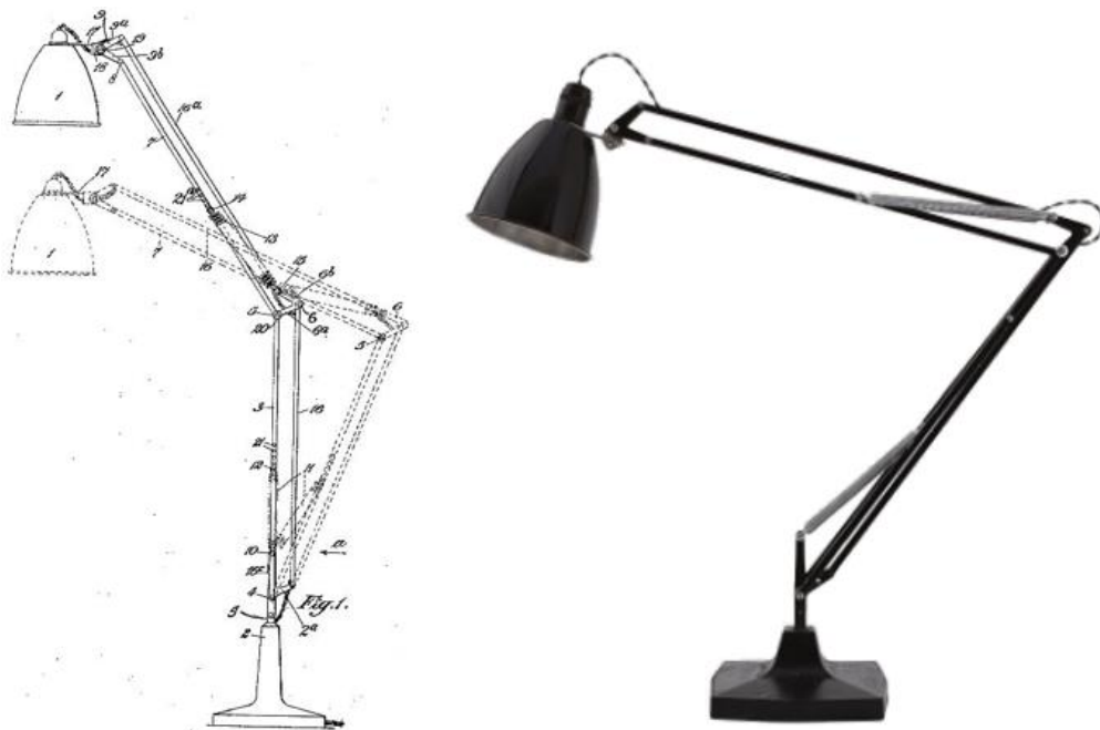
Figure 6. Carwandine's design [14] and Anglepoise Model 1208
