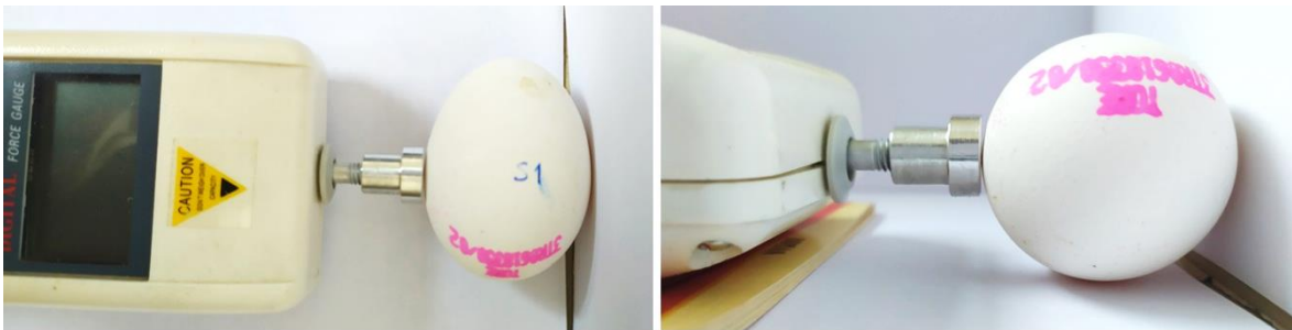
Figure 71. Test setup to determine cracking force
