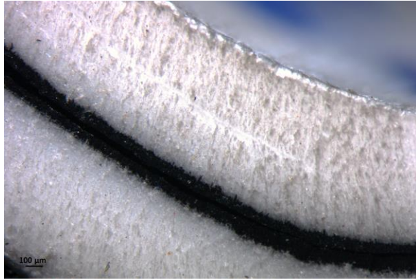
Figure 3.12: Representative optical microscope image for 0.13 and 0.2 wt.% CNT BP reinforced composites after SBS tests at room temperature.
