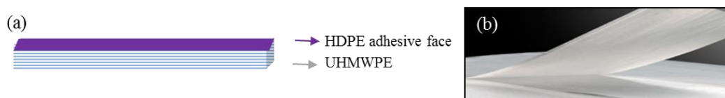
Figure 2.1: Endumax film; (a) schematic illustration, (b) real appearance.
