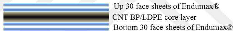
Figure 2.10: Laminated composite design with CNT BP/LDPE core layer in symmetrical face sheet configuration.
