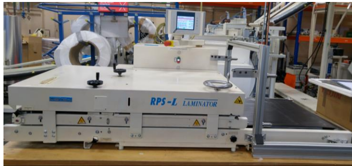
Figure 2.7: Belt laminator for composite fabrication.
