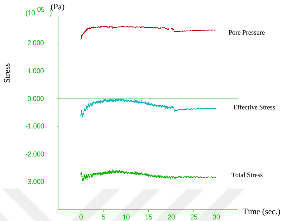
Figure 5.7. Total, effective stress and pore pressure versus time; before the foundation soil improvement.
