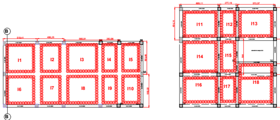
Figure 4.8. Application plan drawings of jet grout cells of I block.
