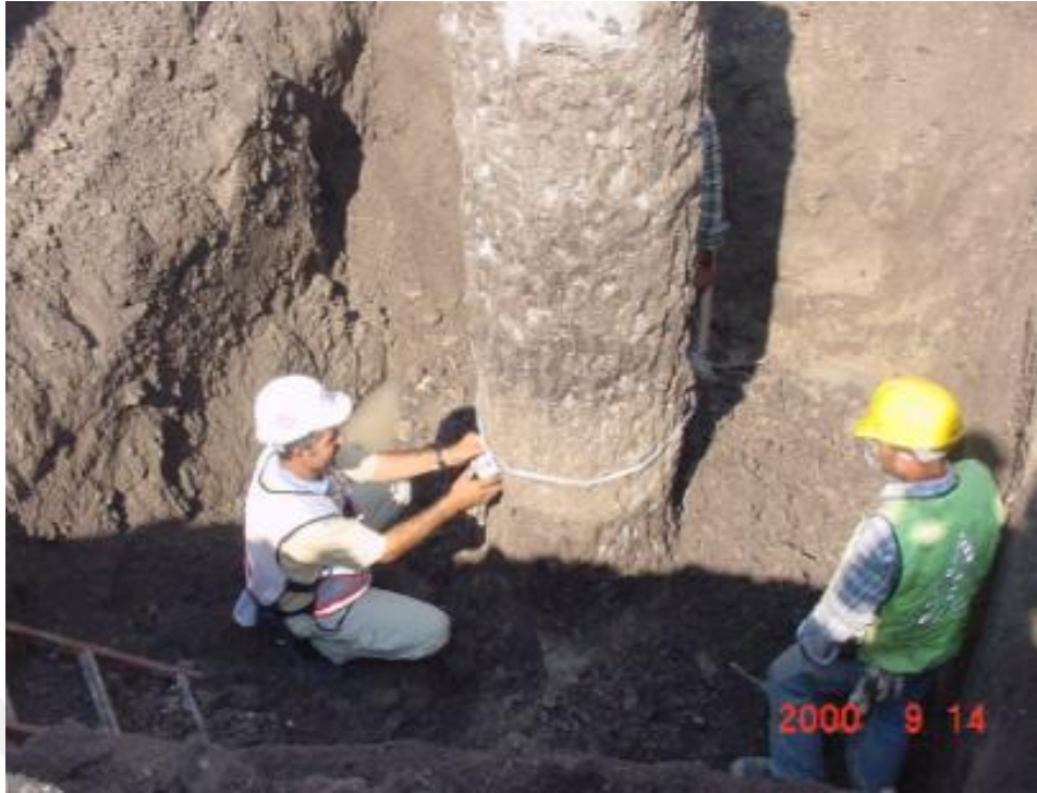
Figure 3.22. Investigation excavation and diameter control of jet grout column (Source: Gökalp and Düzceer 2000).
