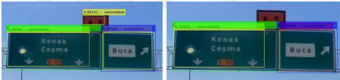
Figure 19. Orange signs before and after adding negative samples in training
