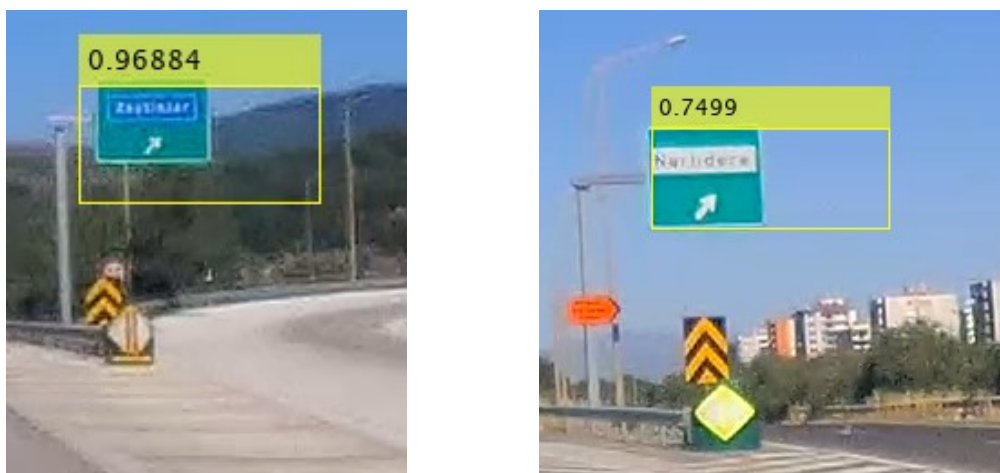
Figure 40. Problem of missized bounding boxes with CNN methods
