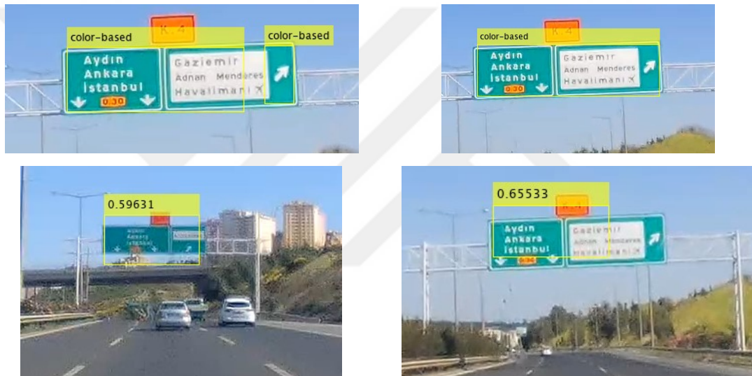
Figure 41. Bounding box problems with both methods
