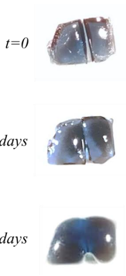
Figure 4.10. Photographs of the Au NP/PAAm composite divided into two pieces. The self-healing feature is shown as a function of time.
