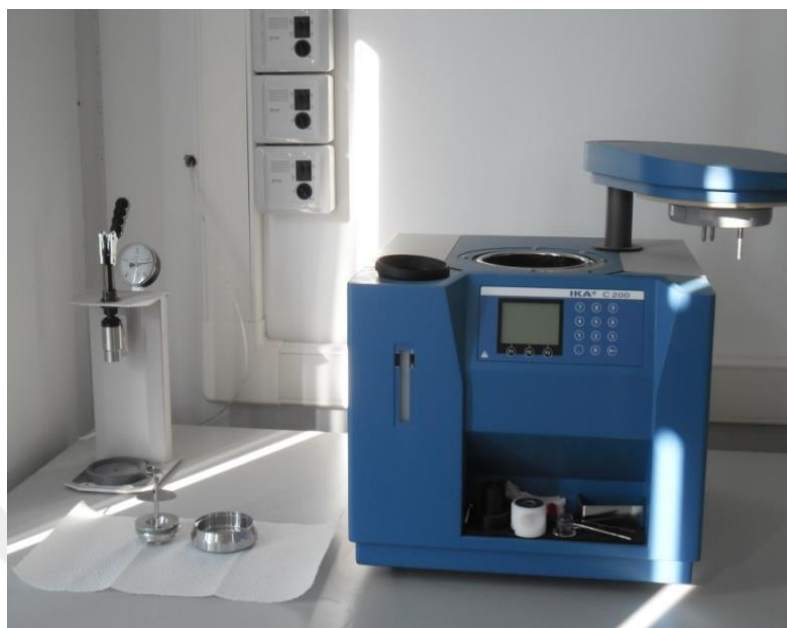
Figure 3.6 Calorimeter used at Aten Brantner Waste Management Co. in which sample collection processes was completed waste acceptance laboratory
