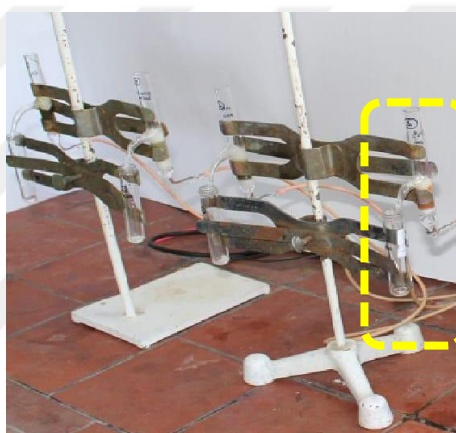
Figure 3.1 Experimental set-up of up-flow fixed bed operation
