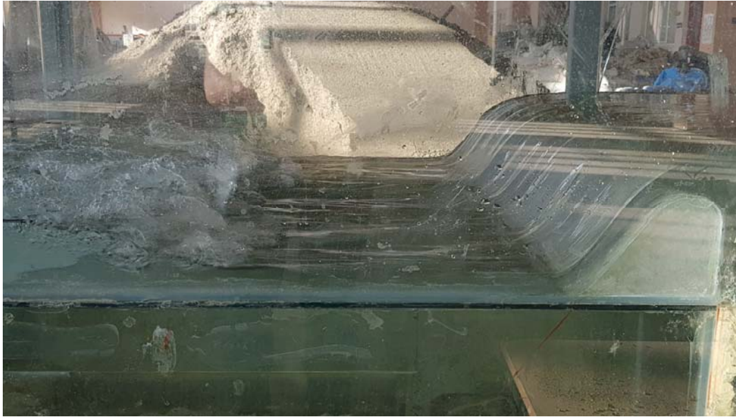
Figure 4.12 Hydraulic Jump formation downstream of the spillway – no blocks case
