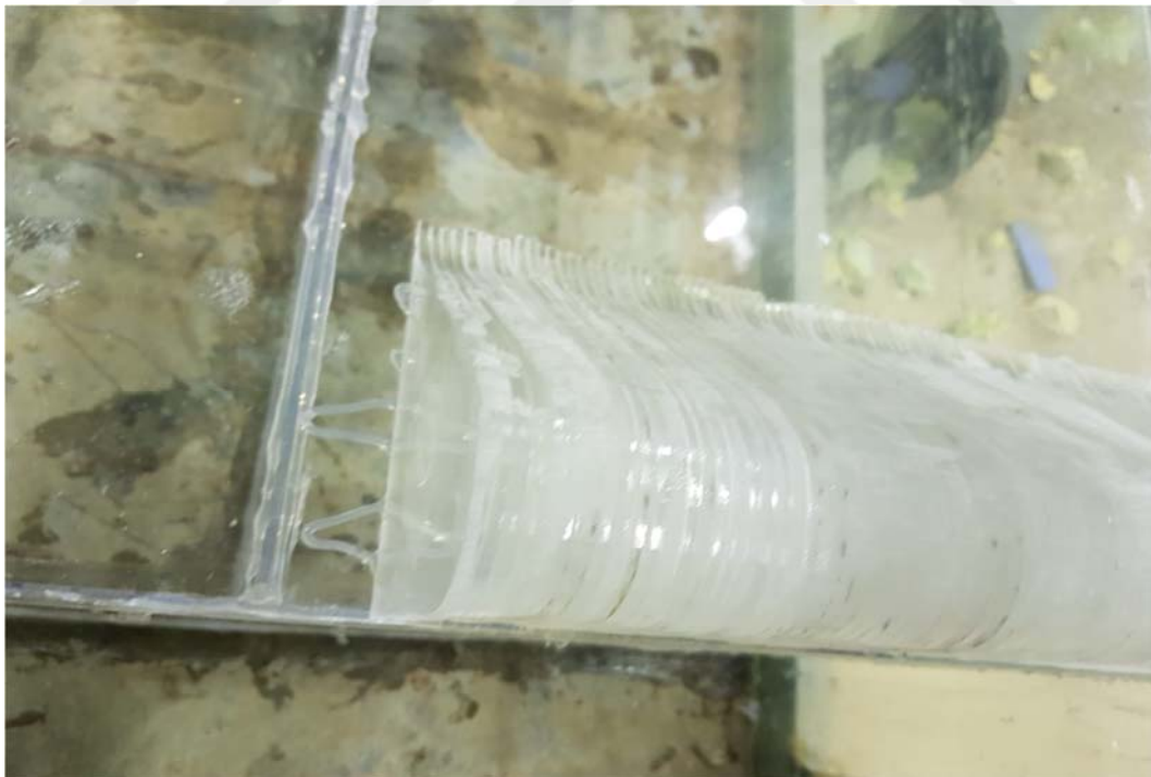
Figure 3.8 The Plexiglas slices of the spillway profile, gathering slices
