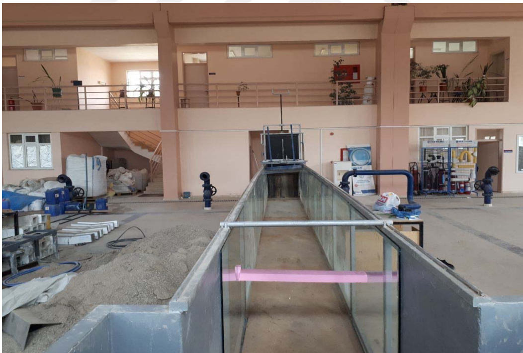
Figure 4.2 Water Flume, Control front gate
