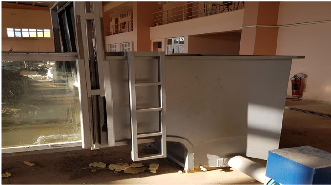
Figure 4.4 Inlet tank of the water flume
