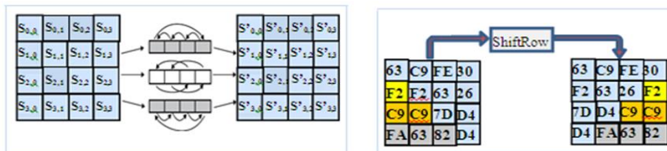
Figure 4.22: ShiftRow Transformation. Figure 4.23: An example of ShiftRow.
