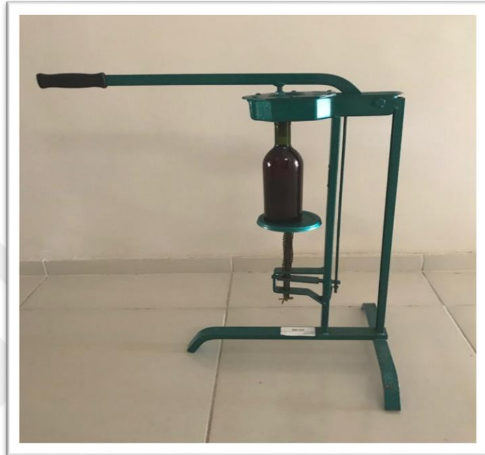
Figure B.1 Cork closure at the semi automatic sealing machine
