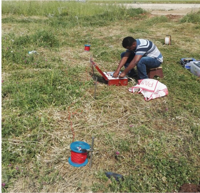
Figure 4.2. Measuring resistivity method at the field
