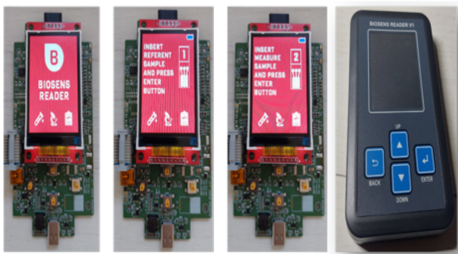
Picture 4.3. The reader circuit for rGO-FET Devices.
