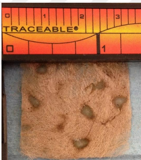
Figure 19. An image of S23/M7/PE70 non-woven hot-pressed at 120°C for 1 min
