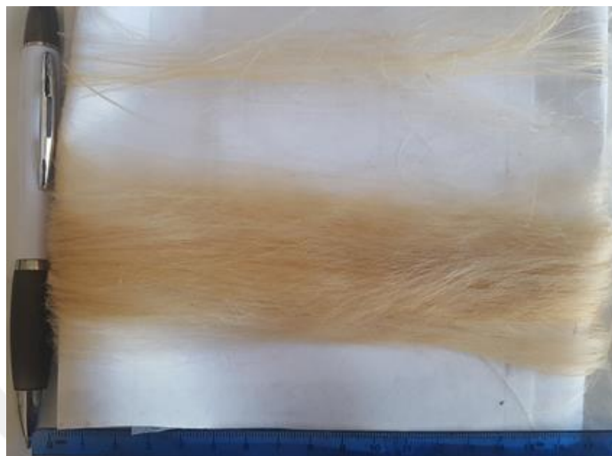
Figure 12. A small roll of soy-PE fibers continuously spun fibers from an S23/M7/PE70 composition
