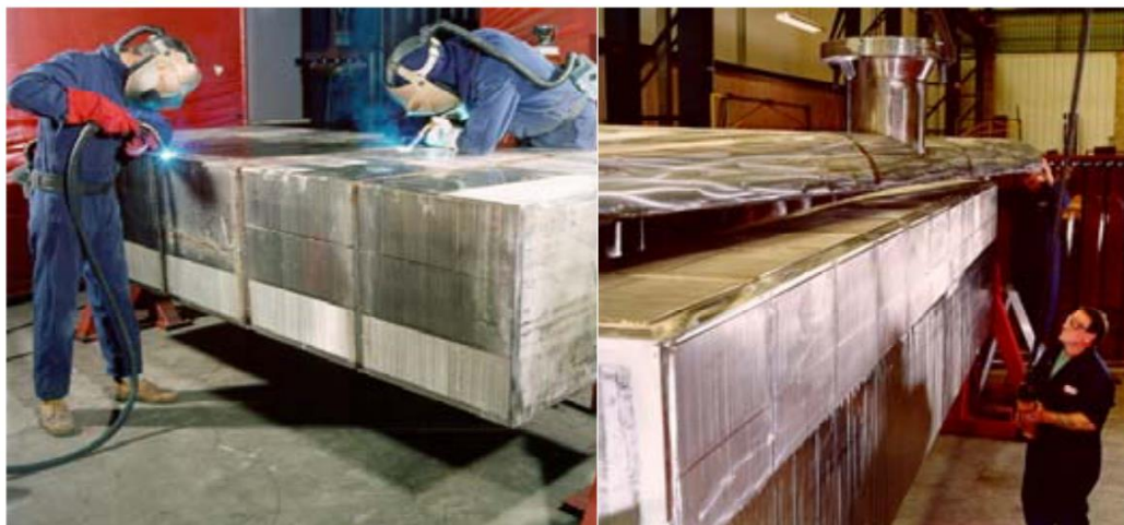
Figure 3.2. The manufacturing process of PFCHEs [13]
