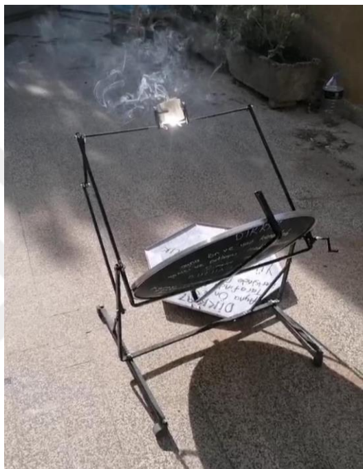
Figure 2-1: Homemade concave mirror system used for solar pyrolysis method.
