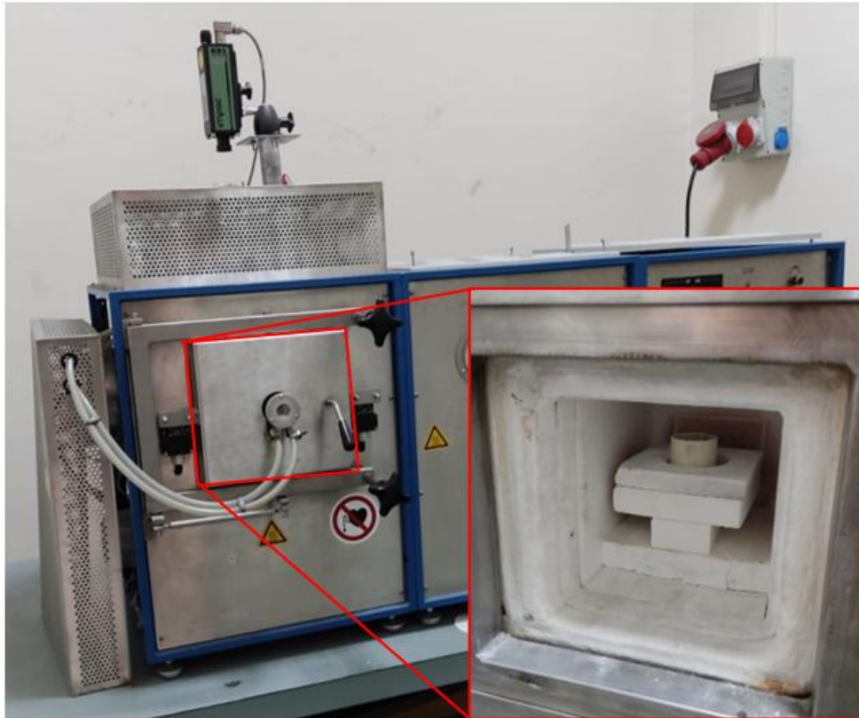
Figure 3.2. Microwave furnace located at the Electromagnetic Materials Laboratory of Metallurgical and Materials Engineering Department of Middle East Technical University.
