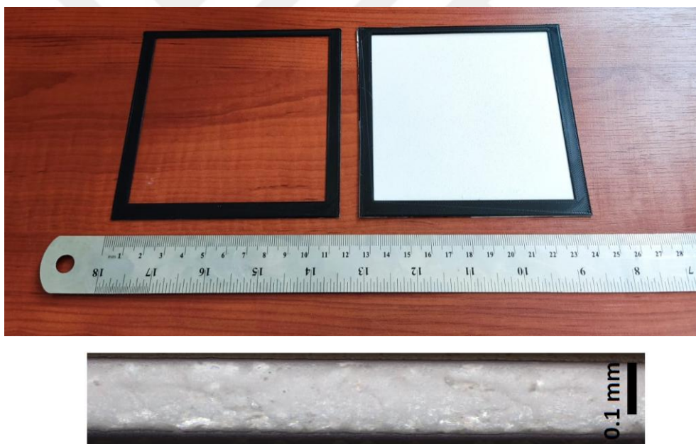
Figure 4.21. (left) 3D printed frame used to attach the BST/ABS films produced via the tape-casting method, (right) the BST/ABS films attached to the 3D printed frame, and (bottom) representative cross-sectional optical image of the tape-casted BST/ABS composite substrate.
