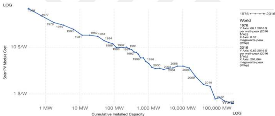
Figure 1.3 Solar PV module prices vs cumulative capacity between 1976 and 2016 [3]
