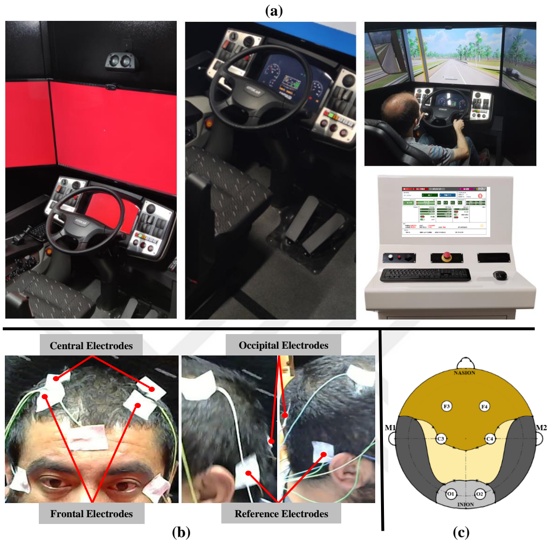
Figure 3. 1: XBUS PRO driving simulator consisting of various training scenarios, camera system, voice communication system, acceleration and brake pedals, steering, automatic and manual transmission, instructor station for remote control and a variety of sensors to record the driving attributes (b) Six-channel EEG device (NOX-A1 system; Nox Medical Inc., Reykjavik, Iceland to record EEG signals at 200 Hz sampling rate (c) International 10-20 system used for the placement of EEG electrodes on the scalp of a subject (F3 and F4: frontal, C3 and C4: central, O1 and O2: occipital, M1 and M2: reference).
