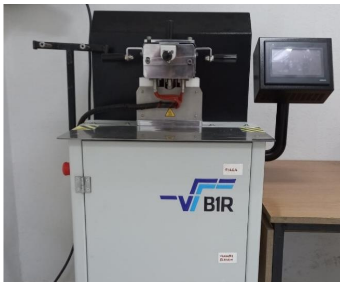
Figure 3.1 : Kökbir RTX-M40 Internal Melt Mixer.
