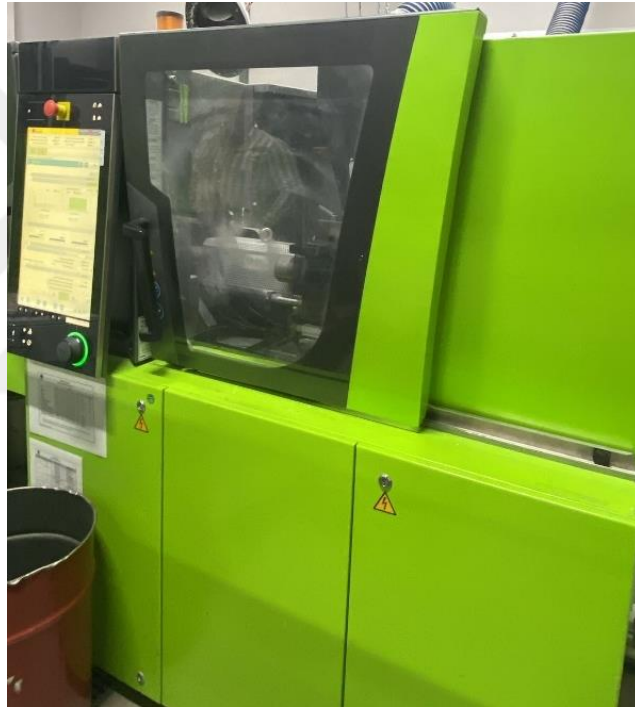
Figure 3.3 : ENGEL victory 50 Injection Molding.
