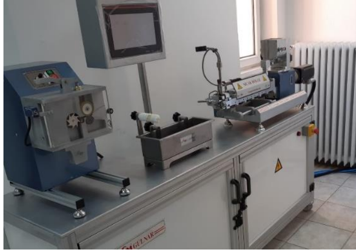
Figure 3.2 : Gülnar GM Twin 16mm L/D 30:1 Twin Screw Extruder.
