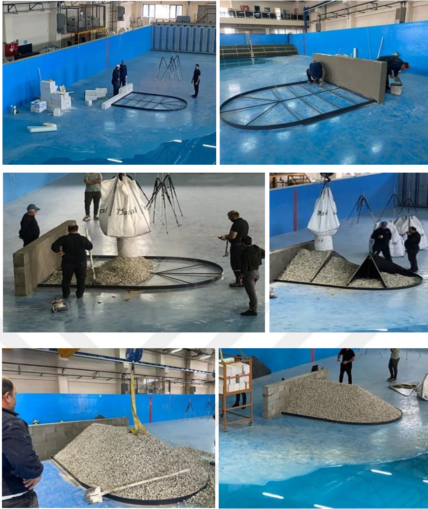
Figure 3.18 Creation of model cross-section
