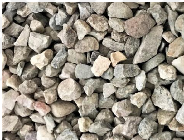
Figure 3.4 Core material of roundhead model
