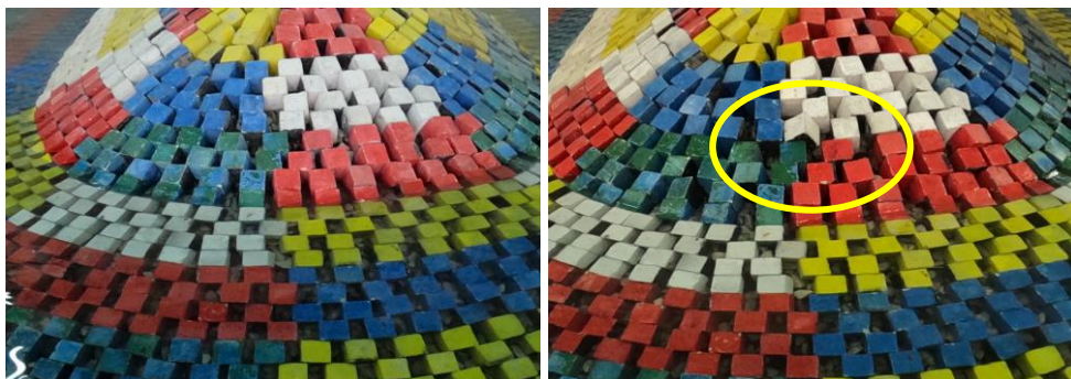
Figure 3.13 Moving blocks after the tests
