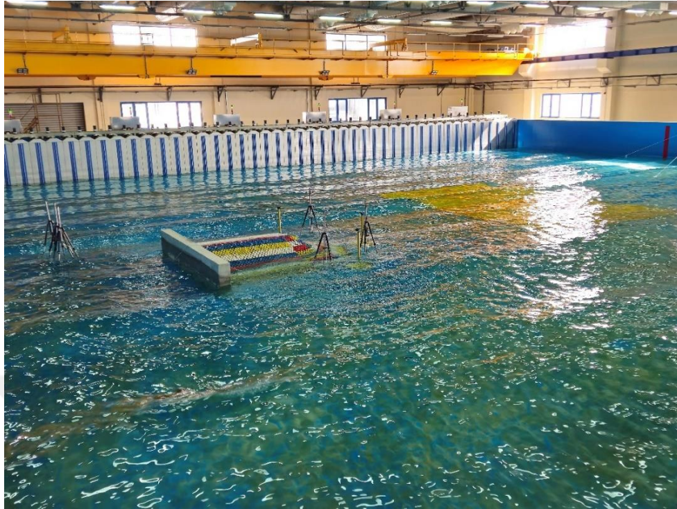
Figure 3.2 General view of wave basin and overhead crane
