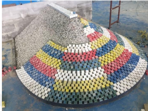
Figure 3.11 Construction phase of the roundhead model
