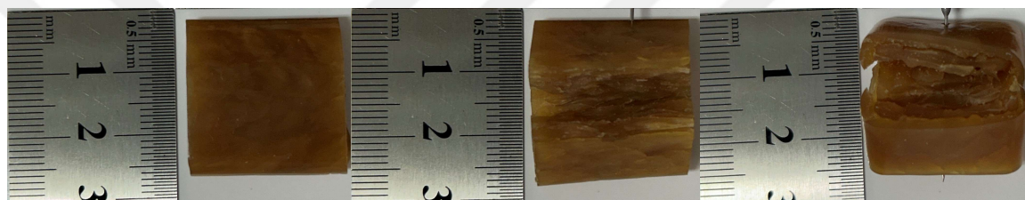
Figure 7: HMMA, H:SPI_0:100, 70% moisture, 100°C. Images of surface, longitudinal to flow and transversal to flow, respectively
