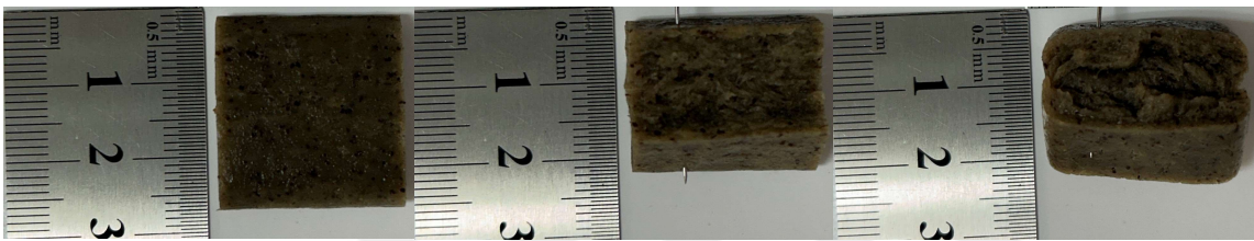
Figure 10: HMMA, H:SPI_25:75, 70% moisture, 100°C. Images of surface, longitudinal to flow and transversal to flow, respectively
