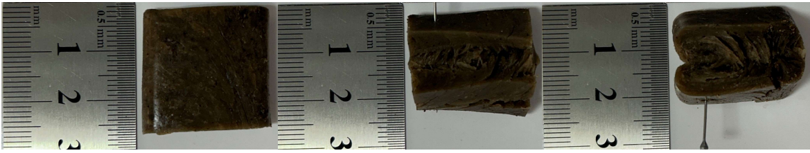
Figure 9: HMMA, H:SPI_25:75, 65% moisture, 100°C. Images of surface, longitudinal to flow and transversal to flow, respectively
