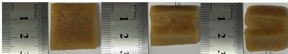
Figure 7: HMMA, H:SPI_0:100, 70% moisture, 100°C. Images of surface, longitudinal to flow and transversal to flow, respectively
