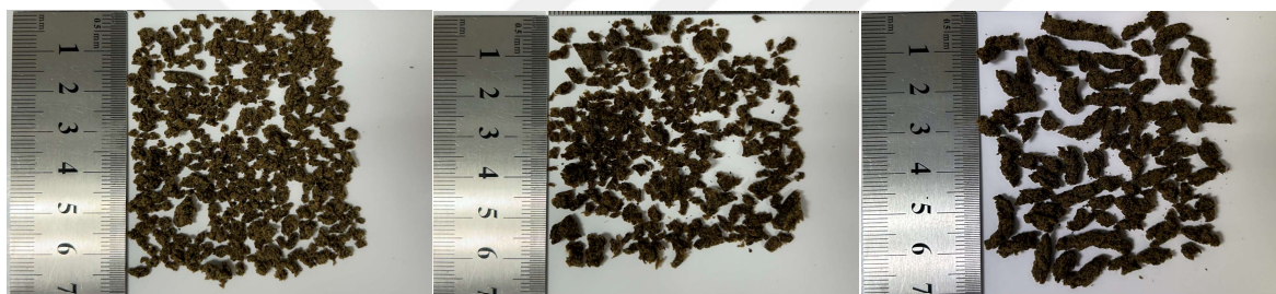
Figure 5: LMMA, H:G_60:40, 20% moisture, 150°C
