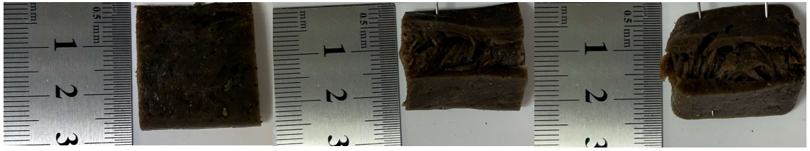
Figure 18: HMMA, H:SPI_25:75, 65% moisture, 125°C. Images of surface, longitudinal to flow and transversal to flow, respectively
