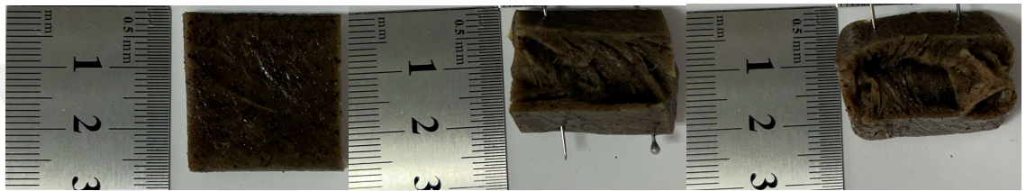
Figure 19: HMMA, H:SPI_25:75, 70% moisture, 125°C. Images of surface, longitudinal to flow and transversal to flow, respectively
