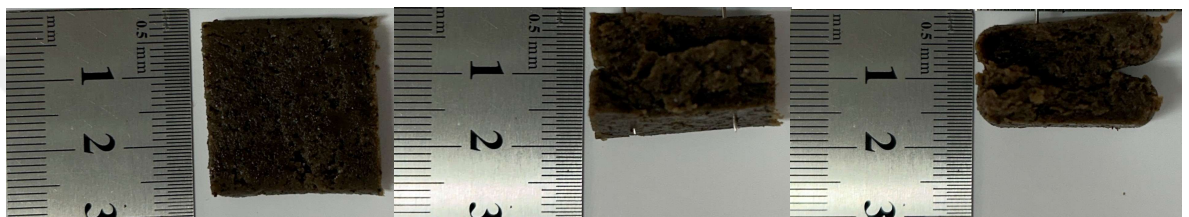
Figure 13: HMMA, H:SPI_50:50, 70% moisture, 100°C. Images of surface, longitudinal to flow and transversal to flow, respectively
