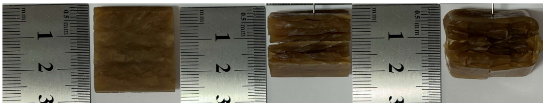
Figure 16: HMMA, H:SPI_0:100, 70% moisture, 125°C. Images of surface, longitudinal to flow and transversal to flow, respectively
